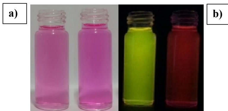
Figure S20: a) Day light photograph image of BOD-ZN + Hg(II) (left), BOD-ZN (right), (b) fluorescence image of BOD-ZN + Hg(II) (left), BOD-ZN (right)
