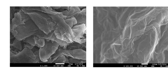
Figure S1. FE SEM images of graphite and few layer graphene used to prepare sulfur composite electrode for high volumetric energy density Li-S batteries
