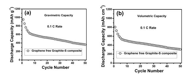
**Figure S4.** Electrochemical performance of graphene free graphite-sulfur composite a) gravimetric capacity (mAh g<sup>-1</sup>) and b) volumetric capacity (mAh cm<sup>-3</sup>)
