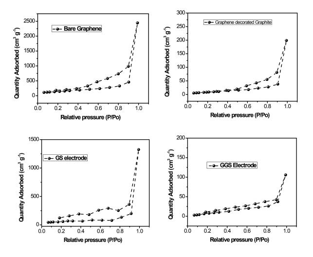
Figure S2. BET surface analysis of bare graphene, graphene - graphite matrix and their composites with sulfur respectively
