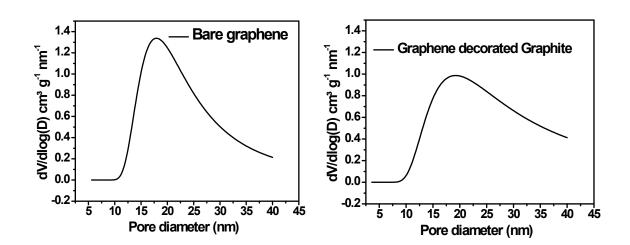
**Figure S3.** Pore size distribution of bare graphene (low tap-density) and graphene - graphite composite (high tap-density)
