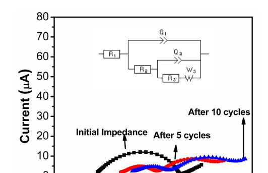
Figure S5. Electrochemical Impedance spectra of uncoated high density GGS electrode vs.  $Li/Li^+$
