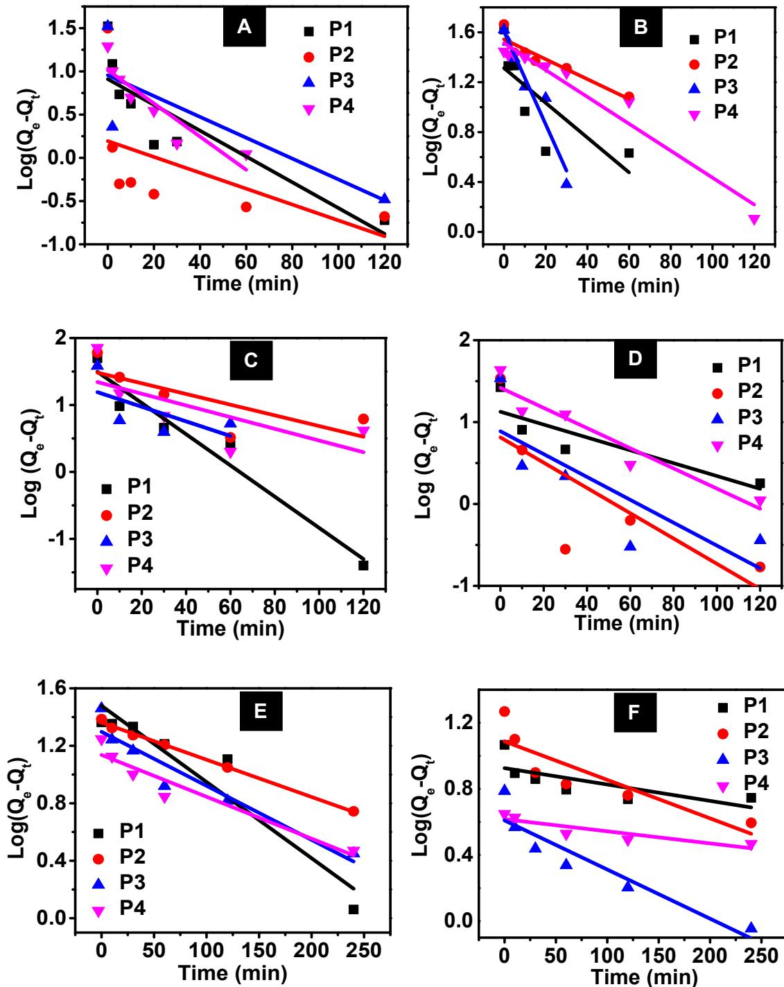
**Figure S2.** Pseudo-first order kinetics for the polymers with (A) Ag-PVP, (B) Au-PVP, (C) Brilliant Blue, (D) Neutral Red, (E) Pb(II) and (F) Cr(VI) ions.
