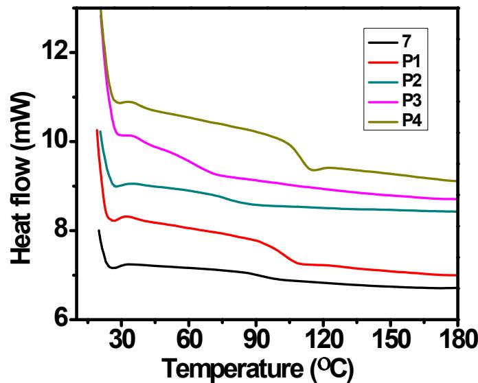
**Figure S1.** DSC curves of random copolymers in nitrogen atmosphere
