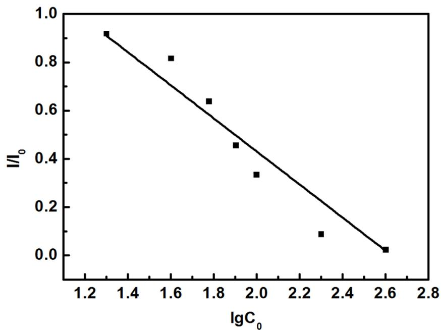
**Fig. S10** The luminescent quenching effect of different concentrations of  $\text{Fe}^{3+}$  can be treated with the Stern-Volmer equation,  $I_0/I = 1 + K_{sv}[Q]$ , where  $K_{sv}$  is the quenching constant and  $[Q]$  is the quencher concentration.
