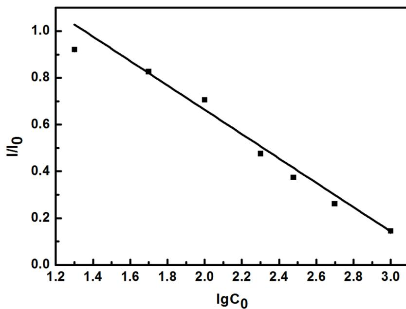
**Fig. S12** The luminescent quenching effect of different concentrations of vitamin C in the water solutions can be treated with the Stern-Volmer equation,  $I_0/I = 1 + K_{sv}[Q]$ , where  $K_{sv}$  is the quenching constant and  $[Q]$  is the quencher concentration.
