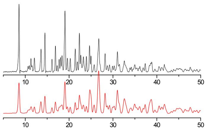
**Fig. S8** Powder X-ray diffraction (PXRD) patterns of the used samples **4** before (black) and after (red) suspending in the analyte solution confirming the integrity of the frameworks.
