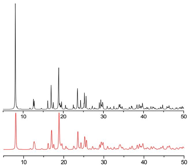
**Fig. S4** Powder X-ray diffraction (PXRD) patterns of **2** (black for calculated and red for experimental ones).
