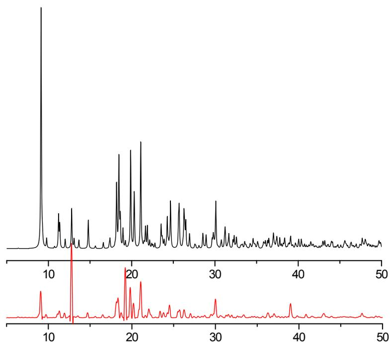
**Fig. S5** Powder X-ray diffraction (PXRD) patterns of **3** (black for calculated and red for experimental ones).
