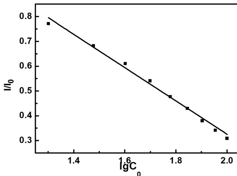
**Fig. S11** The luminescent quenching effect of the different concentrations of actone into the water solutions can be treated with the Stern-Volmer equation,  $I_0/I = 1 + K_{sv}[Q]$ , where  $K_{sv}$  is the quenching constant and  $[Q]$  is the quencher concentration.
