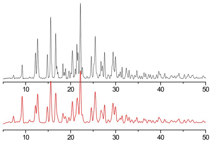
**Fig. S9** Powder X-ray diffraction (PXRD) patterns of the used samples **5** before (black) and after (red) suspending in the analyte solution confirming the integrity of the frameworks.
