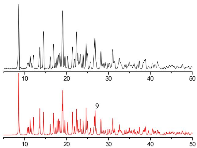
**Fig. S6** Powder X-ray diffraction (PXRD) patterns of **4** (black for calculated and red for experimental ones).
