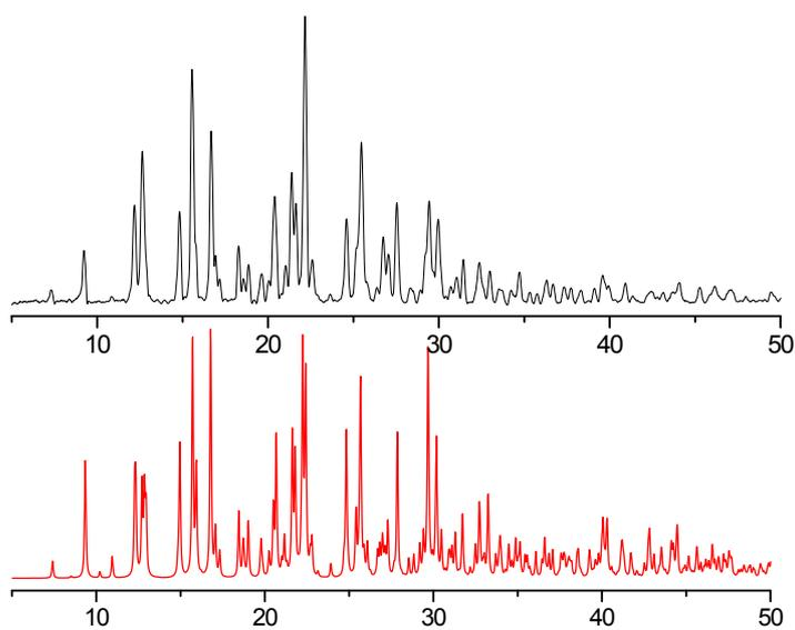
**Fig. S7** Powder X-ray diffraction (PXRD) patterns of **5** (black for calculated and red for experimental ones).
