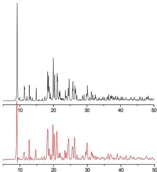
**Fig. S3** Powder X-ray diffraction (PXRD) patterns of **1** (black for calculated and red for experimental ones).
