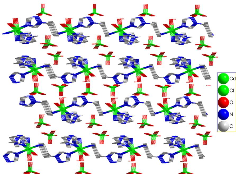
**Fig. S2** 2D coordination micro-porous framework of compound **1**, in which two kinds of different directional free perchlorate anions can be observed between two neighboring layers.
