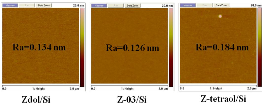
Figure S1 AFM images of PFPE nanofilms on silica surfaces
