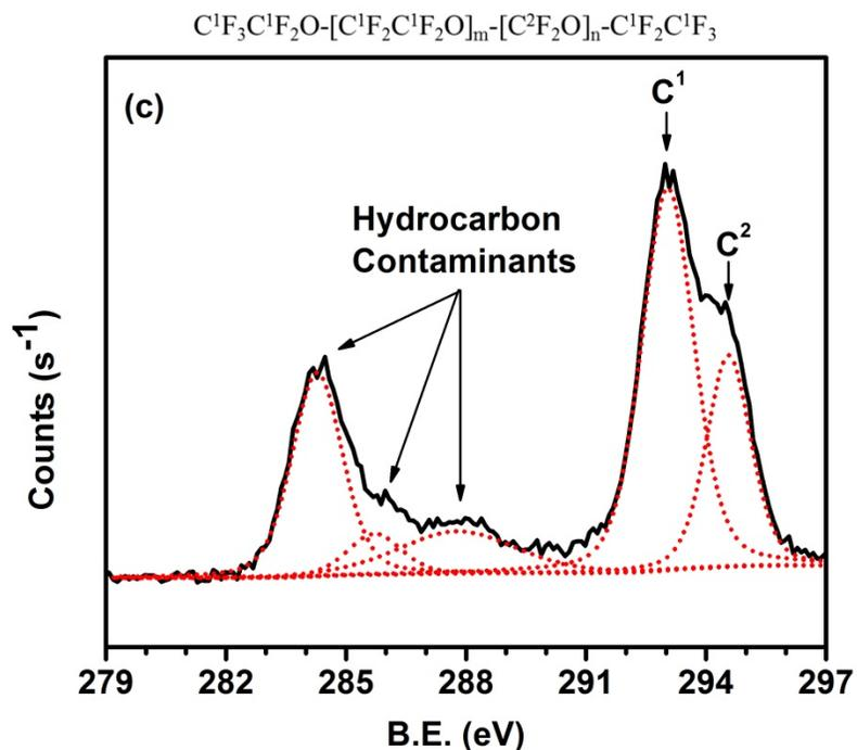
Figure S3 XPS C1s spectra and curve-fitting results (a) Zdol, (b) Z-tetraol, (c) Z-03
