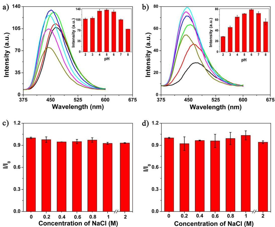
**Figure S1** Effect of pH and salt concentration on the fluorescence of the as-synthesized C-Dots. (a, c) for fraction 1 (AR-C-Dots) and (b, d) for fraction 2 (CR-C-Dots).
