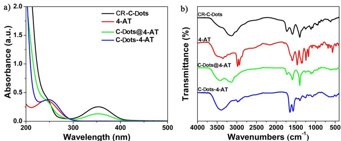
**Figure S4** UV-vis absorbance (a) and FT-IR spectrum (b) of C-Dots-4-AT
