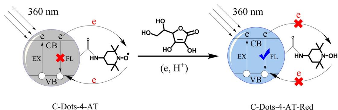
**Scheme S1** Proposed mechanism of ESR and fluorescence dual-responsive nanoprobe of C-Dots-TEMPO for ascorbic acid by Guo et al.<sup>1</sup>
