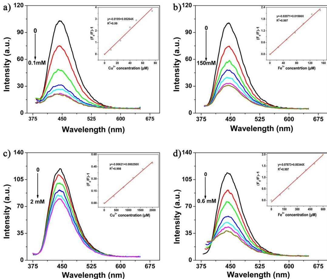
**Figure S2** Fluorescence quenching behaviors of as-synthesized C-Dots by  $\text{Cu}^{2+}$  (a, c) and  $\text{Fe}^{3+}$  (b, d). Conditions: excitation at 360 nm;  $F_0$  and  $F$  are fluorescence intensities at 405 nm in the absence and presence of  $\text{Cu}^{2+}/\text{Fe}^{3+}$ , respectively. (a, b) fraction 1 (AR-C-Dots) and (c, d) fraction 2 (CR-C-Dots).
