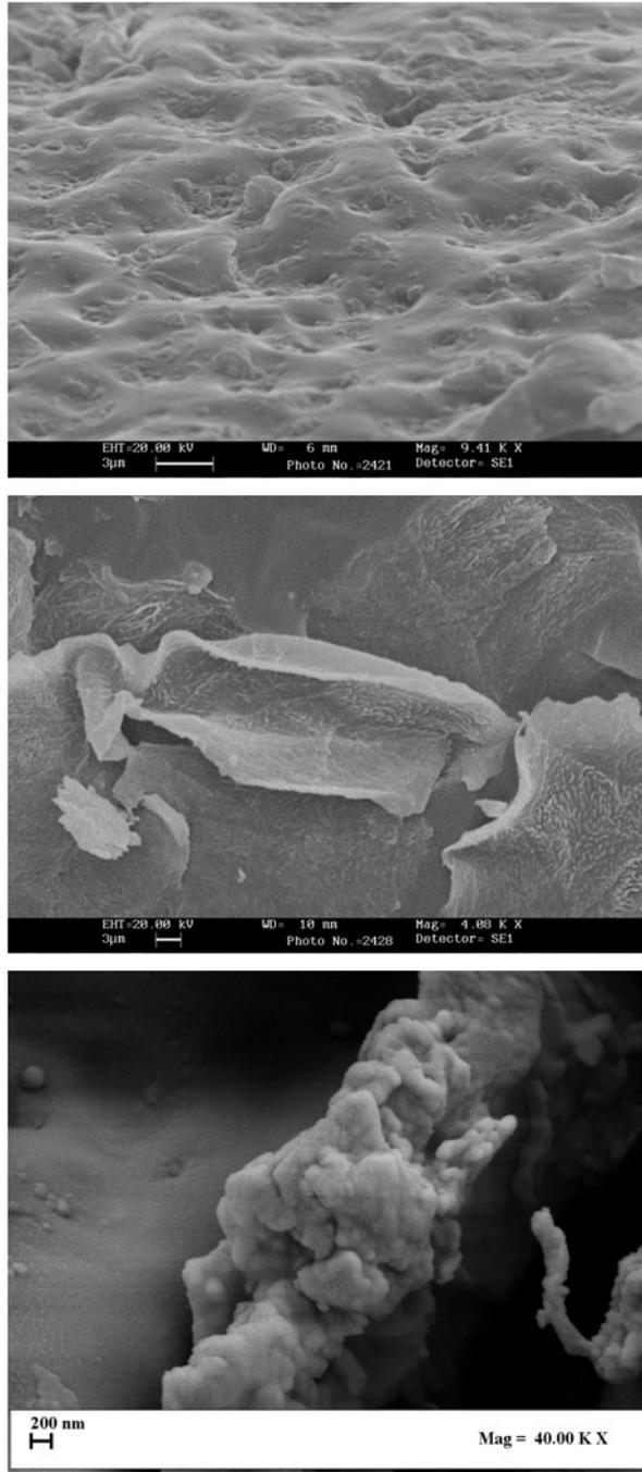
**Figure 7S.** SEM images at different magnification of the fracture surface of nanofilled resin at loading rate of 0.5 % by weight of SL sample.
