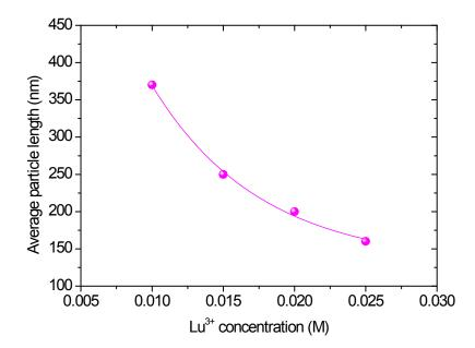
Average particle length versus concentration of Lutetium acetate used in the synthesis of LuPO<sub>4</sub> particles. The rest of synthesis conditions are identical to those given in Figure 1 of the paper.
