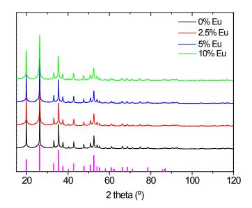
XRD patterns of LuPO<sub>4</sub> nanoparticles doped with different Eu<sup>3+</sup> contents
