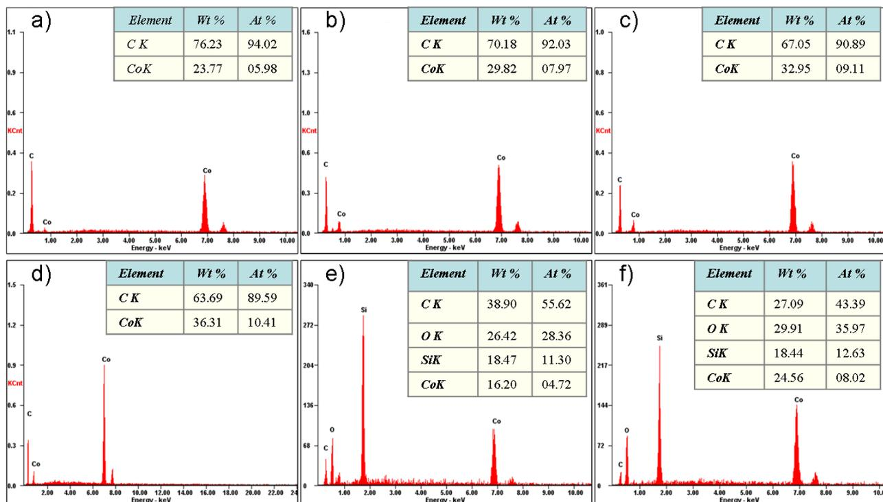
**Figure S4.** SEM-EDX spectra of the materials obtained through thermolysis of compounds: a) T-700-8h, b) T-700-24h, c) T-800-8h, d) T-850-8h, e) PT-700-24h and f) PT-850-8h.
