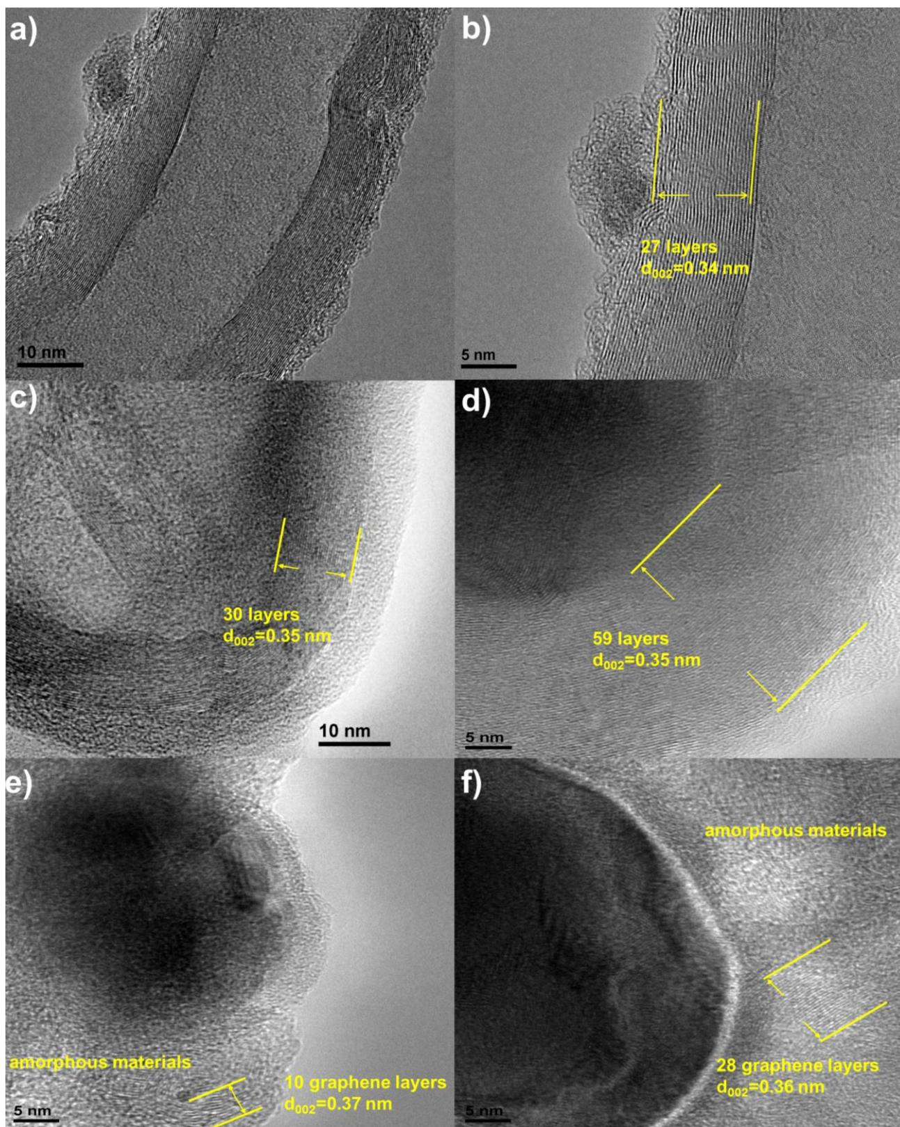
**Figure S3.** HRTEM images of the materials obtained through thermolysis of **T** and **PT**. (a, b) for **T-700-24h**; (c, d) for **T-850-8h**; (e) for **PT-700-24h**; (f) for **PT-850-8h**.
