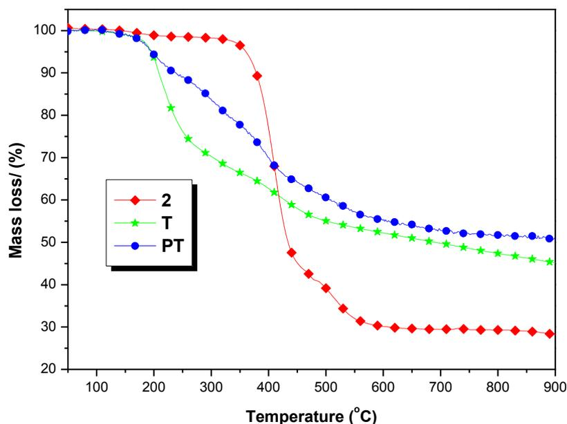
**Figure S2.** TGA thermograms of **2**, **T** and **PT** measured under nitrogen at a heating rate of  $10\text{ }^{\circ}\text{C min}^{-1}$ .
