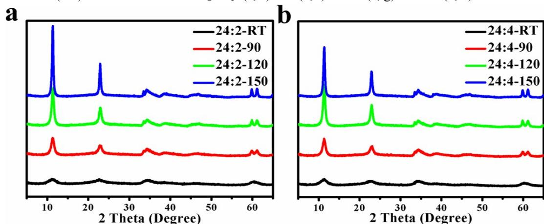
**Fig S2.** The XRD spectra of NiFe-LDH aged under different resultant temperature with a 24:2 (a) and 24:4 (b) ratio of NaOH and Na<sub>2</sub>CO<sub>3</sub>. (c)The partial enlarged view of XRD spectra of NiFe-LDH with a 24:0 ratio of NaOH and Na<sub>2</sub>CO<sub>3</sub>.
