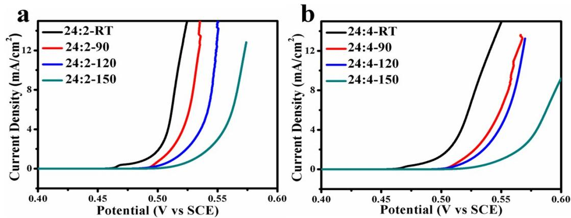
**Fig S3.** The electrochemical performance of NiFe-LDH with (a) 24:2 and (b) 24:4 ratio of NaOH and Na<sub>2</sub>CO<sub>3</sub> respectively.
