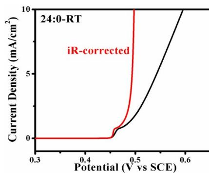
**Fig S6.** LSV curve for modified GC electrodes comprising the 24:0-RT NiFe-LDH with (red) and without (black) correction for iR loss.
