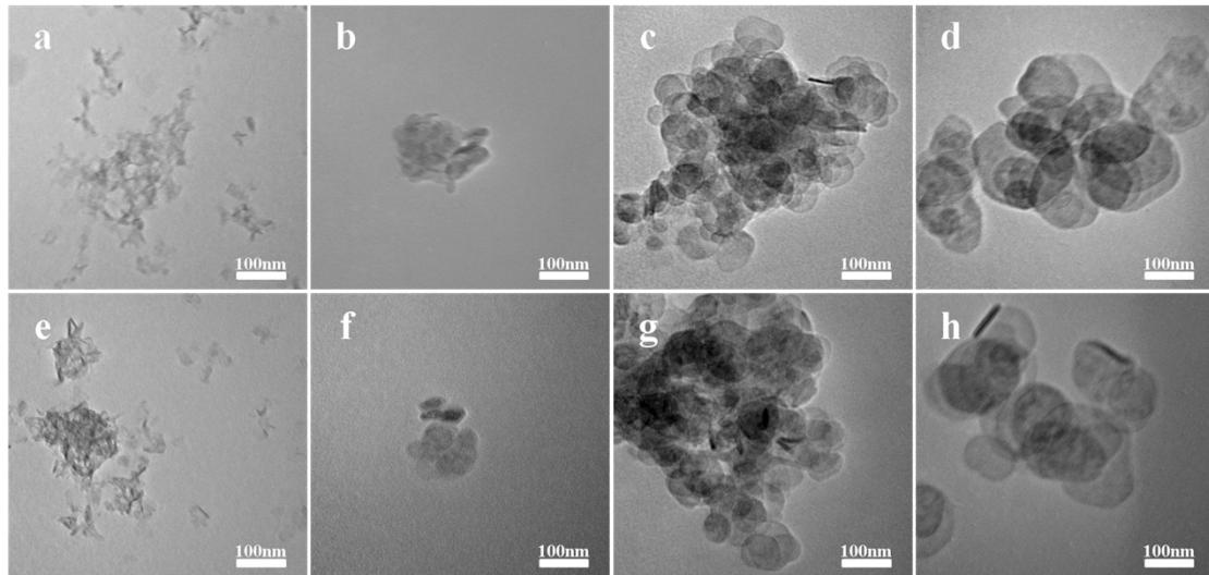
**Fig S1.** TEM images of NiFe-LDH under different resultant temperature for 12 h with a 24:2 (a-d) and 24:4 (e-h) ratio of NaOH and Na<sub>2</sub>CO<sub>3</sub>. (a, e) RT. (b, f) 90 °C. (c, g) 120 °C. (d, h) 150 °C.
