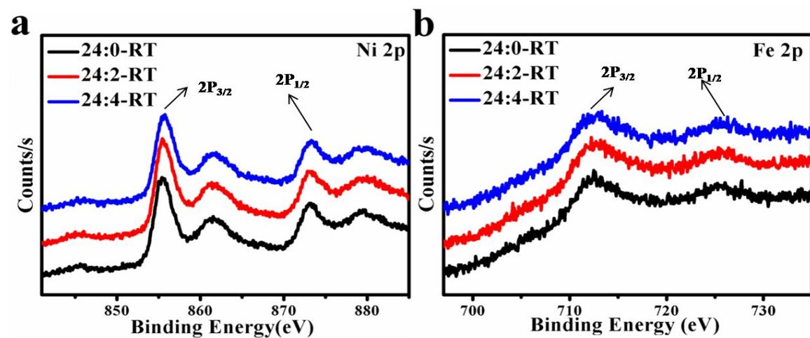
**Fig S5.** The high-resolution (a) Ni 2p XPS survey spectra and (b) Fe 2p XPS survey spectra.
