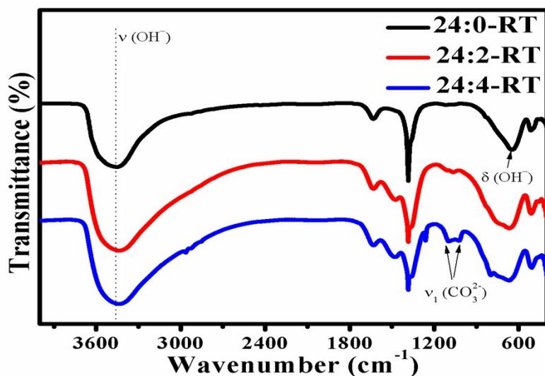
**Fig S4.** The FT-IR spectrum of NiFe-LDH OER catalyst with various ratios of NaOH and Na<sub>2</sub>CO<sub>3</sub> at RT from 4000 to 400 cm<sup>-1</sup>. The labeled v (OH<sup>-</sup>), δ(OH<sup>-</sup>) and ν<sub>1</sub> (CO<sub>3</sub><sup>2-</sup>) are according to *J. Mater. Sci.*, 2003, 38(9): 2087-2093; *J. Raman Spectrosc.* 2008, 39: 582–586 and *J. Bone. Miner. Res.*, 2001, 16(5): 893-900.
