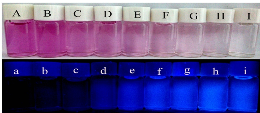
Fig. S8. Color fading (up) and fluorescence increasing (down) of probe 1 ( 5.0 \mu\text{M} ) with the gradual addition of \text{CN}^- (from left to right: 0 \mu\text{M} , 2.0 \mu\text{M} , 4.0 \mu\text{M} , 6.0 \mu\text{M} , 8.0 \mu\text{M} , 10.0 \mu\text{M} , 12.0 \mu\text{M} , 14.0 \mu\text{M} ).
