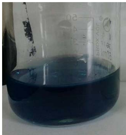
Fig. S7 The solution color of \text{Fe}^{3+} with \text{Na}_2\text{S}_2\text{O}_3 as reductant with the presence of \text{H}_3\text{PMo}_{12}\text{O}_{40}
