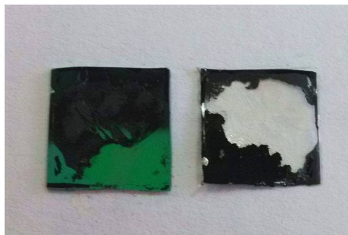
Fig. S1 Photographs of VACNT arrays transferred onto PET substrate with CNTs residues left on silicon substrate.
