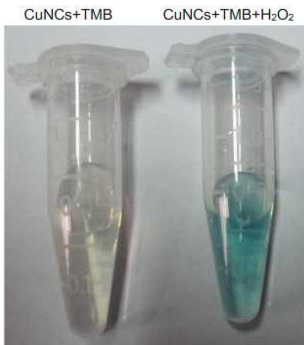
Figure S6 The oxidation of TMB (0.2 mM) in the absence (A) or presence (B) of  $\text{H}_2\text{O}_2$  (10 mM) catalyzed by the small CuNCs ( $174 \mu\text{g mL}^{-1}$ ).
