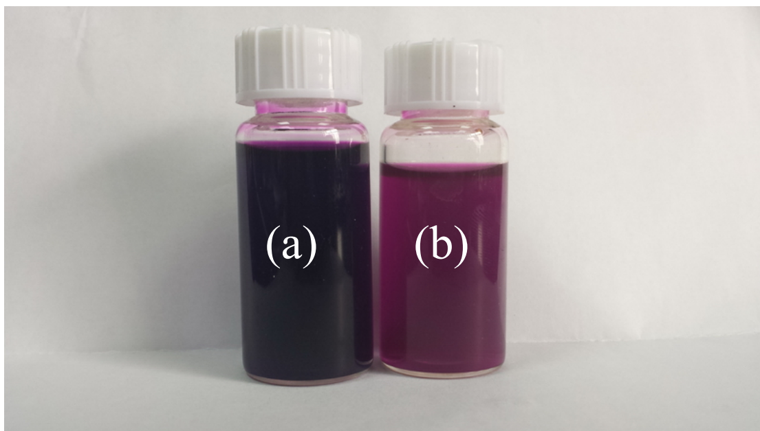
Fig. S3 The color of solution after reaction: initial synthesis solution pH = 7.0 (a) and pH = 1.0 (b).
