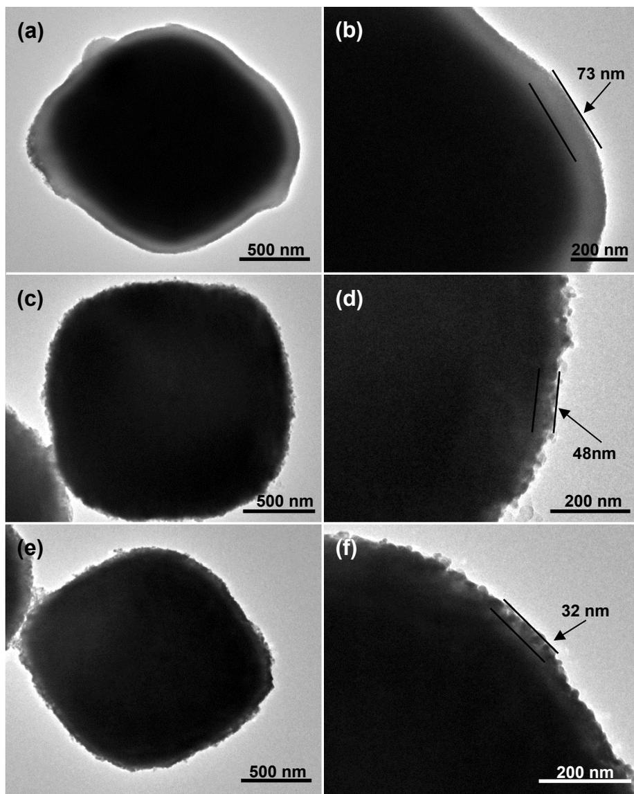
**Figure S1.** High-magnification TEM images of the S-40, S-80, S-120 with a-TiO<sub>2</sub> layers of different thickness( S-40:a, b; S-80: c, d; S-120:e, f).
