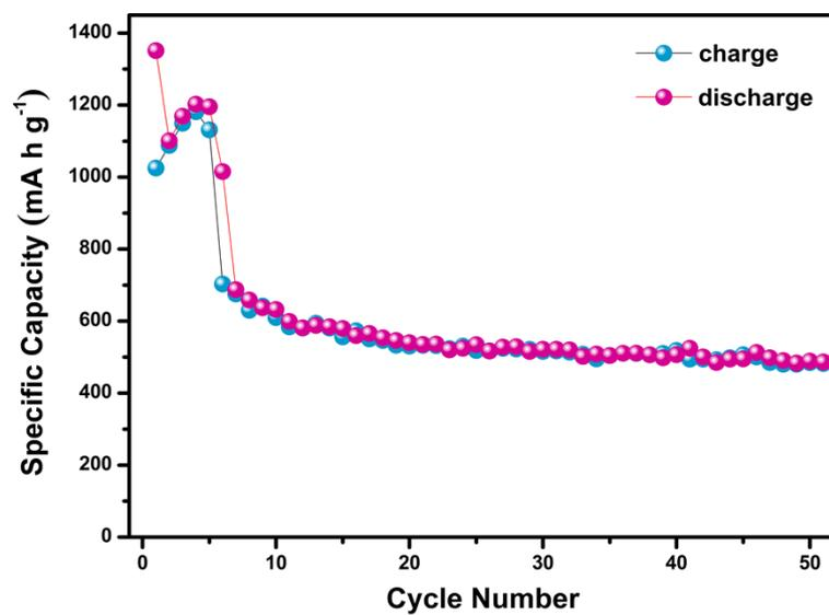
**Figure S6.** Cycle performance of S-80 at a current density of 2 A g<sup>-1</sup>.
