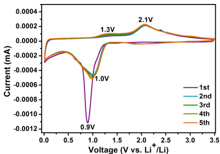
**Figure S4.** Cyclic voltammetry (CV) curves for the S-0 at a scan rate of 0.1  $\text{mV s}^{-1}$  in the voltage windows of 0.01-3.5 V.
