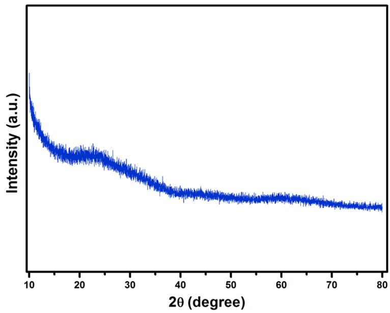
**Figure S2.** XRD pattern of the a-TiO<sub>2</sub>.
