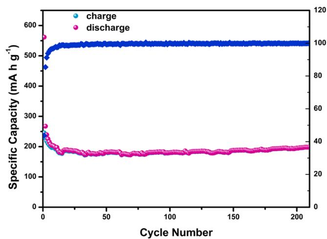
**Figure S7.** Charge-discharge curves of a-TiO<sub>2</sub> at a current density of 0.5 A g<sup>-1</sup>.
