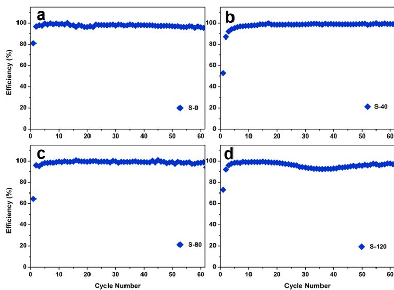
**Figure S5.** The Coulombic efficiency for the samples (S-0: a; S-40: b; S-80: c; S-120: d).
