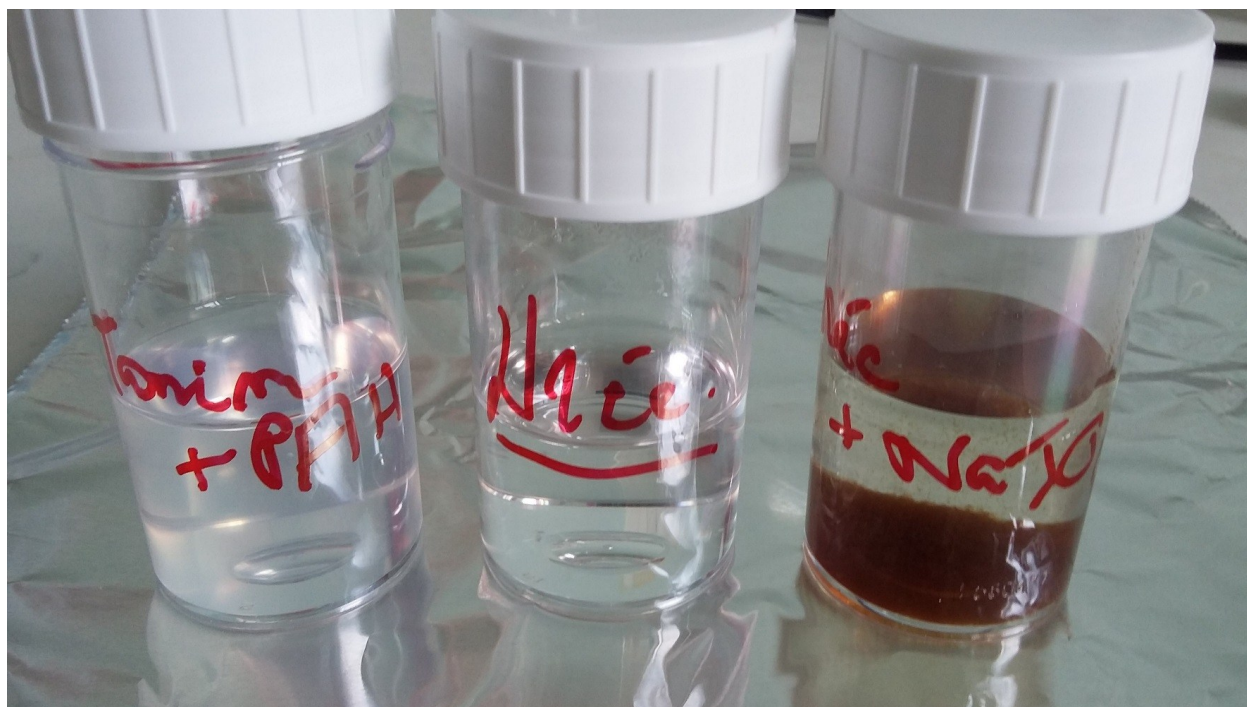
Figure SI4: From the left to the right: digital pictures of a PAH-TA mixture, the PAH-TA mixture put in the presence of a 1 M NaCl-1M urea containing sodium acetate buffer, and the PAH-TA mixture put in the presence of 10 mM NaIO 4 (during 5 min) before subsequent addition of the NaCl-urea containing buffer. The total concentration of TA and PAH was the same in the three bottles. For more details see the Materials and Methods section in the main article.
