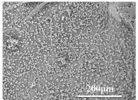
SEM image of C4G8: The pore surface appeared rough and disorder in C4G8, many tiny gelatin particles adhered uniformly on the surface of material.
