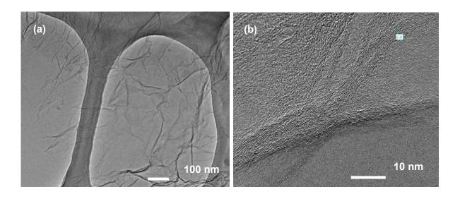
Fig. S1. (a) Low resolution and (b) high resolution TEM images of pristine graphene.
