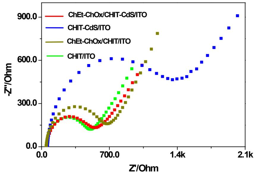
**Figure S3**-Impedance spectra of CHIT/ITO(green),ChEt-ChOx/CHIT/ITO (dark yellow), CHIT-CdS/ITO (blue), and ChEt-ChOx/CHIT-CdS/ITO (red) in PBS (7.4 pH) containing  $[\text{Fe}(\text{CN})_6]^{3-/4-}$  as a redox species.
