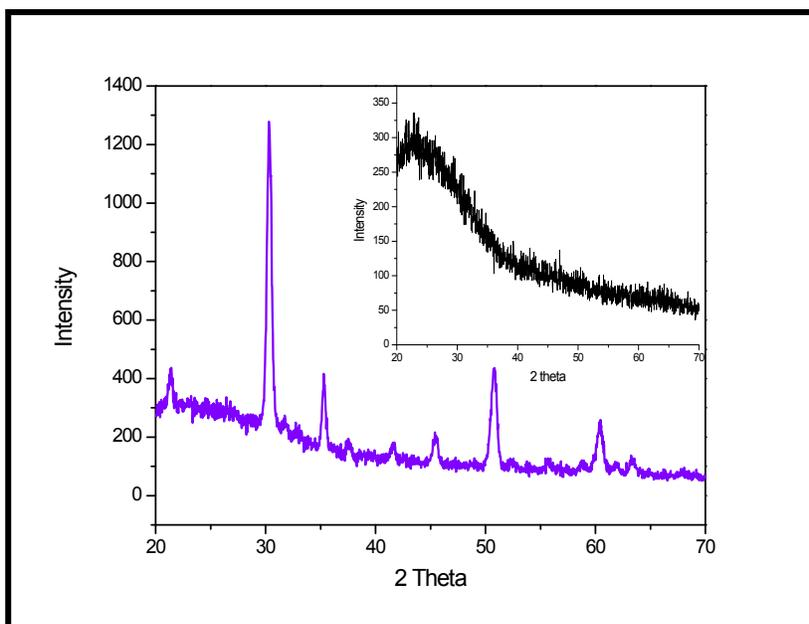
**Figure S1:** XRD pattern of Chitosan film (inset) and CHIT-CdS (QDs) composite film.
