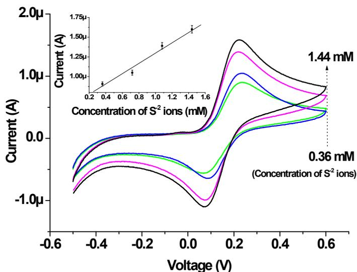
**Figure S2:** CV of the ChEt-ChOx/CHIT-CdS/ITO as a function of  $\text{S}^{2-}$  ions (inset: anodic current vs concentration of  $\text{S}^{2-}$  ions)
