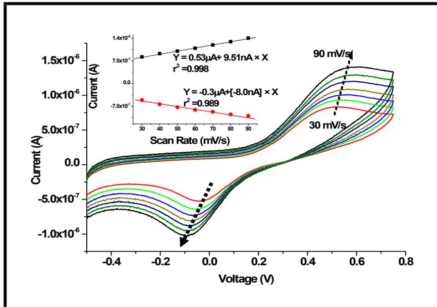
**Figure S4:** Cyclic voltammetric (CV) of ChEt-ChOx/CHIT-CdS/ITO bioelectrode at different scan rate 30-90 mV/s in PBS (50mM, pH7.4, 0.9% NaCl) solution.
