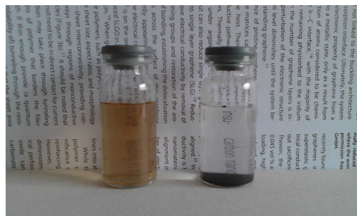
Fig. S1 Optical images of GO (a) and Eu-GO (b) after their dispersions with 1 h sonication stand for 10 h.
