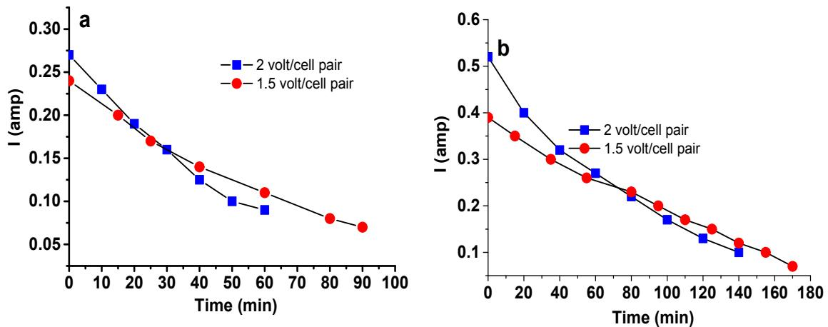
**Fig. S1.** Variation of  $I$  (amp) with time during diluted sea water desalination containing TDS (a) 2000 and (b) 5000 mg/L respectively with CEM-3 at 1.5-2 volt/cell pair applied potential.
