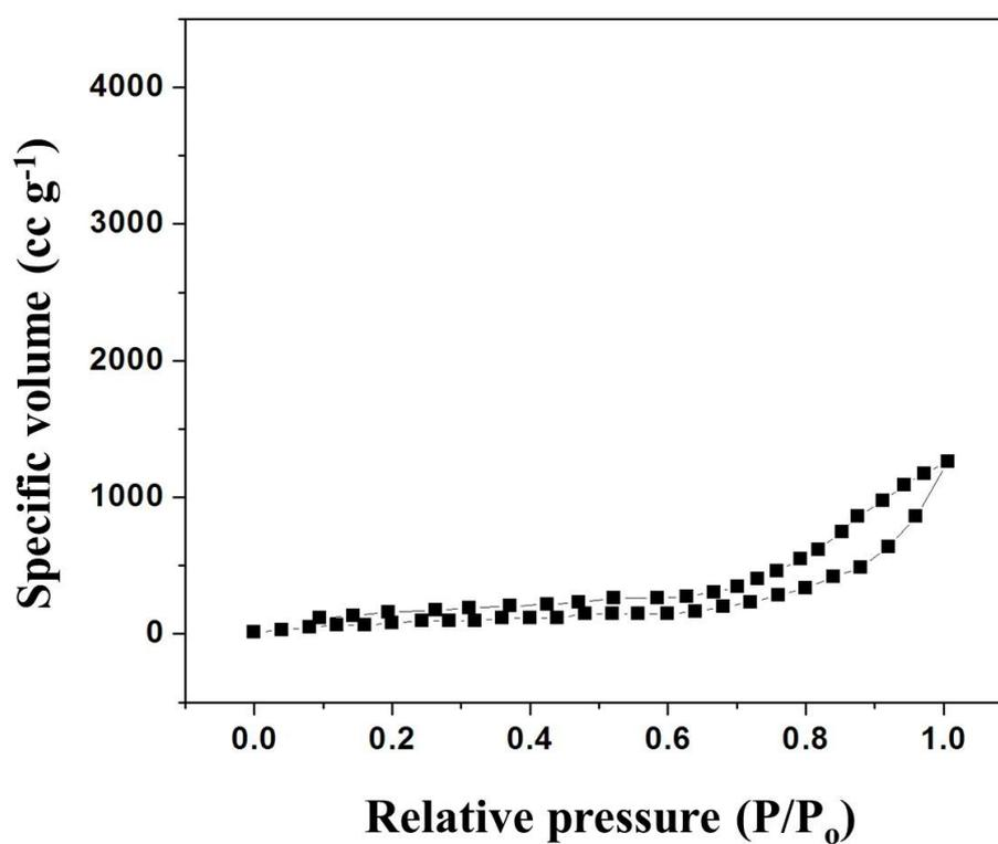
**Fig. S1** Nitrogen adsorption-desorption isotherm of pure CP materials without activation of KOH.
