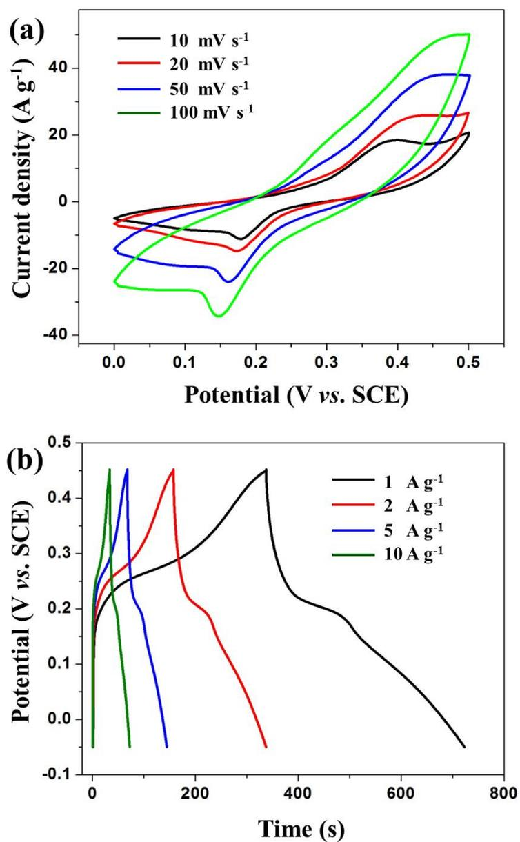
**Fig. S2** CV curves at various scan rates from 10 to 100  $\text{mV s}^{-1}$  (a) and galvanostatic charge-discharge curves at current densities of 1, 2, 5, 10  $\text{A g}^{-1}$  for sample of non-activated CP materials loaded with same content of NiAl-LDHs as that of sample CP/LDH-5.
