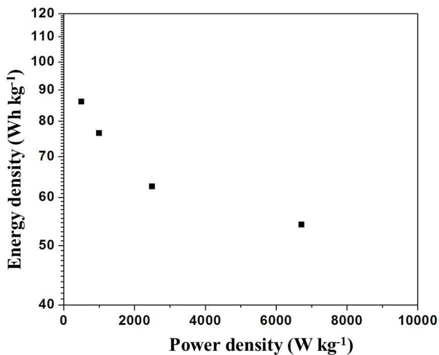
**Fig. S4** Ragone plots of energy density *versus* power density for the CP/LDH-5 sample acting as active electrode material.
