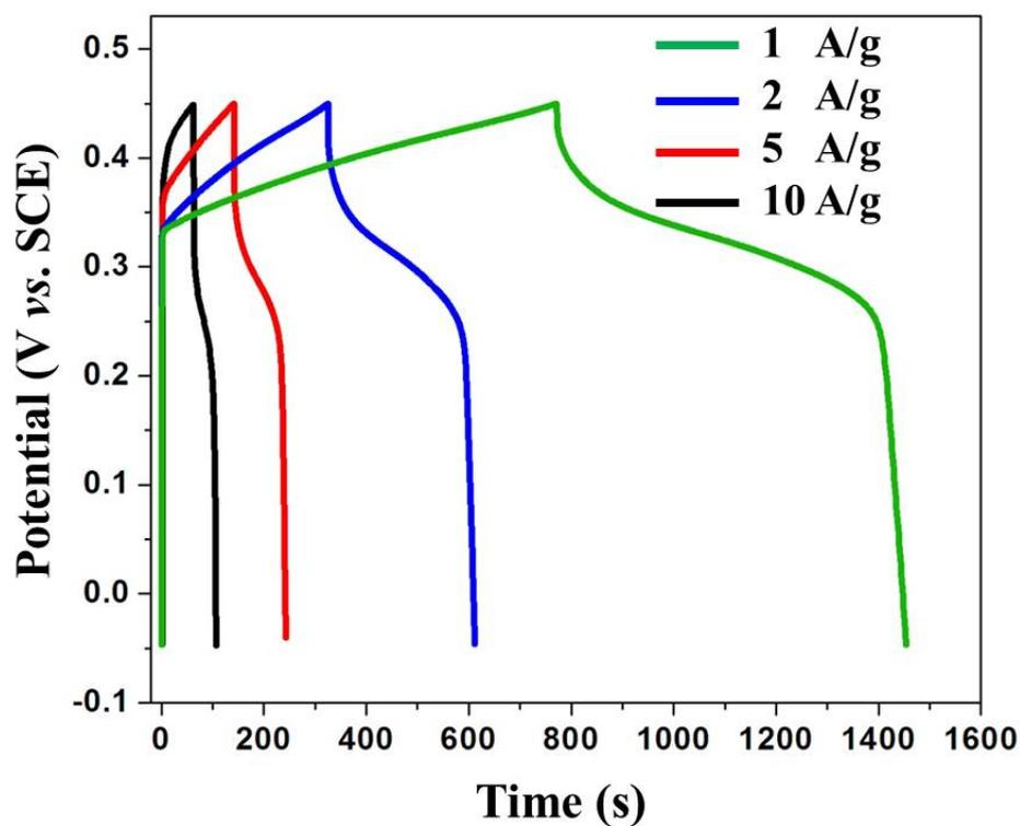
**Fig. S3** Galvanostatic charge-discharge curves at current densities of 1, 2, 5, 10 A/g for sample CP/LDH-5.
