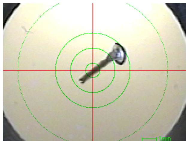
Fig 3a. Sample G12, dimensions under the minimum required for EDXRF analysis at the used equipment (Shimadzu model EDX 700).
