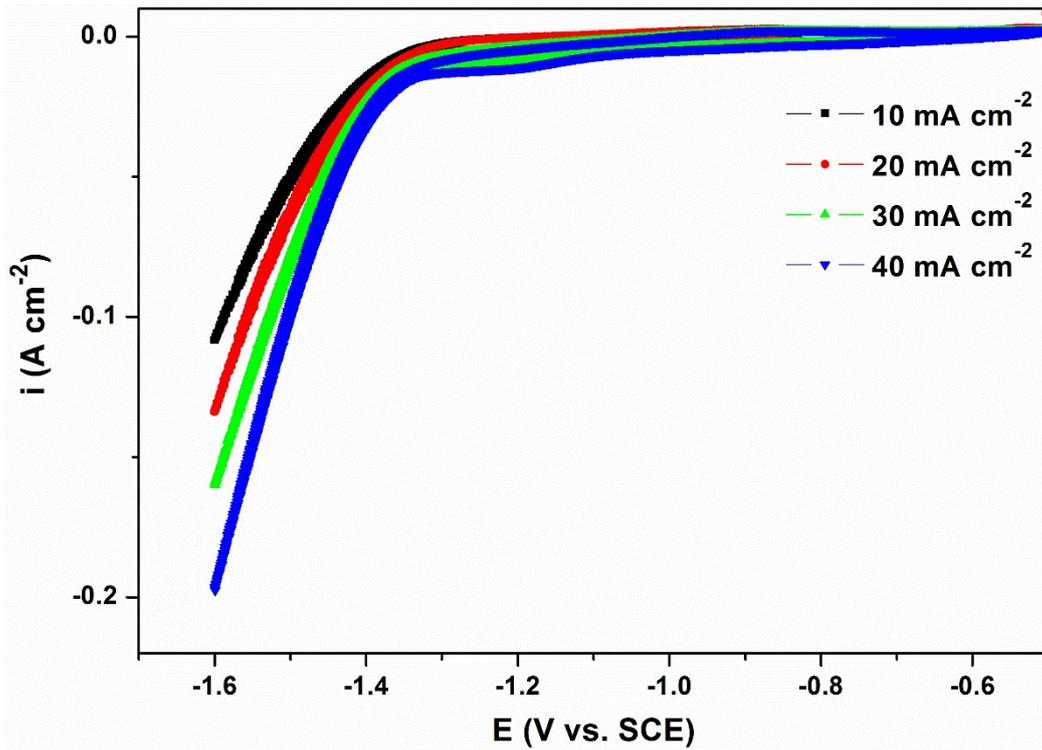
Fig. 5 CV curves showing the peak current density ( $i_{pc}$ ) attained at the end of 50<sup>th</sup> cycle on Co-Ni alloy coatings deposited on copper substrate at different current densities.
