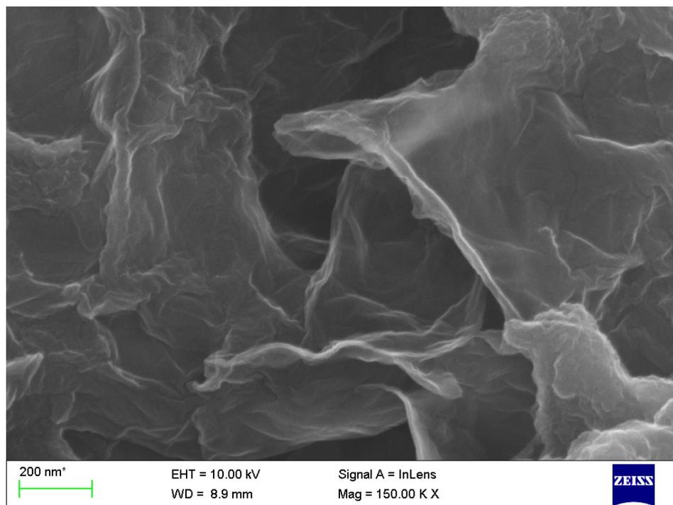
Fig. 1 High magnification FESEM image showing graphene nanosheets.
