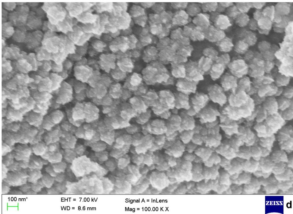
**Fig. 2** Surface morphology of Co-Ni alloy coatings deposited at different current densities: a)  $10 \text{ mA cm}^{-2}$ , b)  $20 \text{ mA cm}^{-2}$ , c)  $30 \text{ mA cm}^{-2}$  and d)  $40 \text{ mA cm}^{-2}$  displaying different degree of surface roughness.
