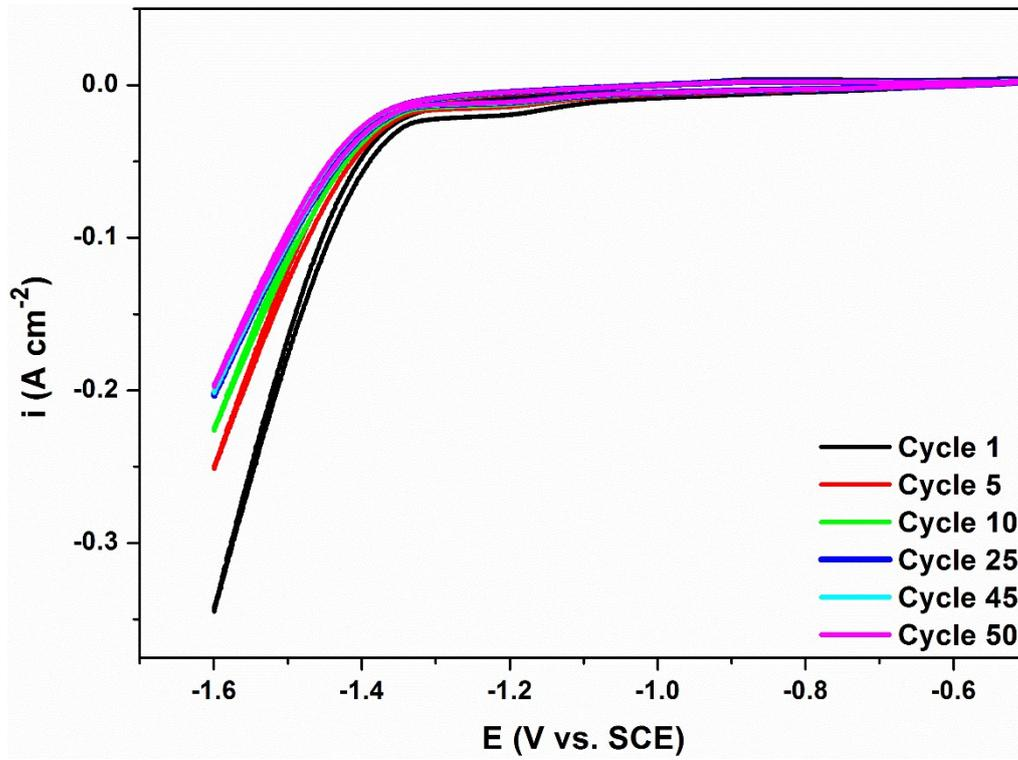
**Fig. 4** CV curves for HER on Co-Ni coating developed at  $40 \text{ mA cm}^{-2}$  in 6 M KOH showing an increase in  $i_{pc}$  with the number of cycles and stabilization after 25<sup>th</sup> cycle.
