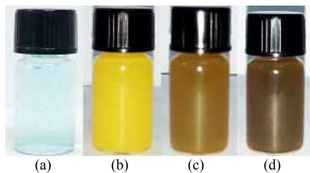
Fig. S4 The photographs showed the color of the solution with the extension of reaction time. (a) 5 min after adding NaOH to CuCl 2 solution, (b) 5 min after adding AA to the solution, (c) 15 min and (d) 30 min after adding N 2 H 4 ·H 2 O to the solution.
