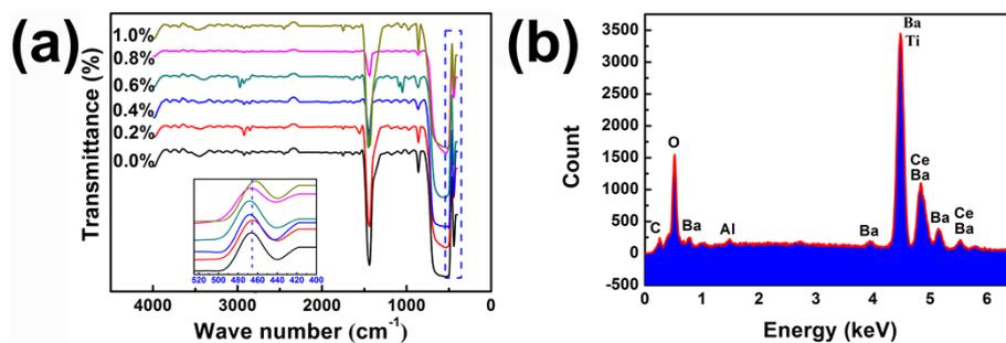
Figure S5 (a) FTIR spectra of Ce-doped BTO nanofibers with different cerium concentration. The broad band at  $3400\text{ cm}^{-1}$  is assigned to the asymmetric vibration of O-H stretching of water molecules adsorbed.
