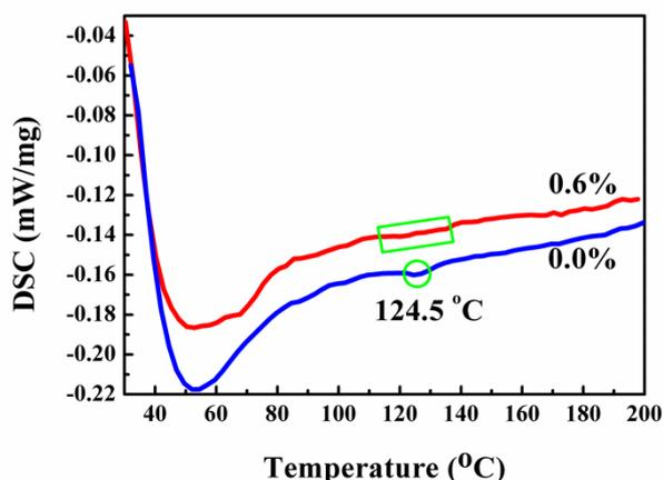
Figure S6 Differential scanning calorimetry (DSC) curves of the BTO nanofibers with Ce/Ba atomic ratios of 0.0% and 0.6%, respectively.
