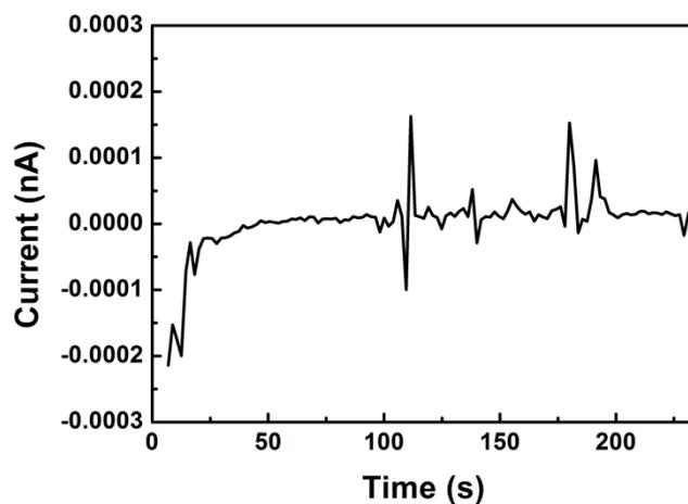
Figure S3 Output current of the energy harvester which contain no BTO nanofibers
