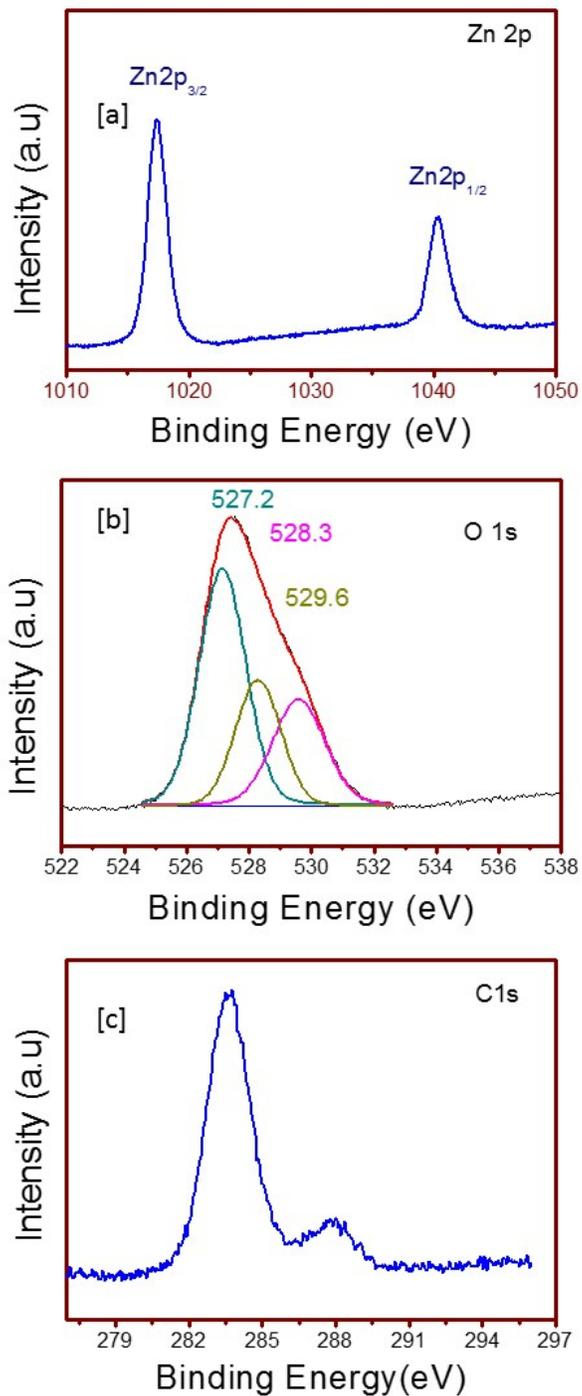
Figure S1. High resolution (a) Zn 2p, (b) O 1s and (c) C 1s core level XPS spectra of CQD/N-ZnO.
