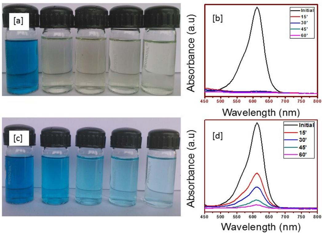
Figure S6. Photographs and UV-Vis absorbance spectra of MG dye degradation in presence of (a-b) CQD/N-ZnO and (c-d) N-doped ZnO photocatalysts, under 0, 15, 30, 45, and 60 min of daylight irradiation.
