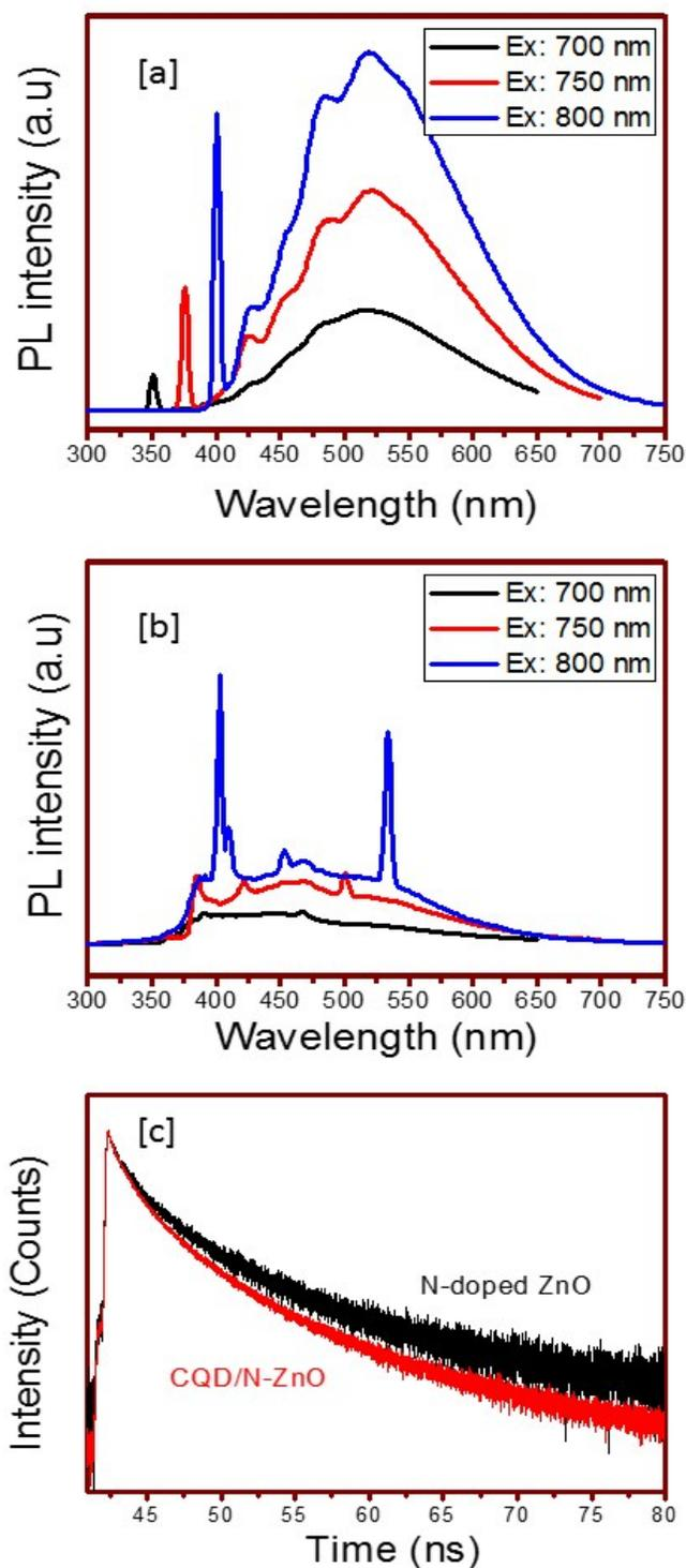
Figure S5. The up-conversion PL emission spectra of (a) pure CQD and (b) CQD/N-ZnO photocatalysts under different excitation wavelength. Time resolved PL spectra of (c) pure N-doped and CQD/N-ZnO photocatalysts.
