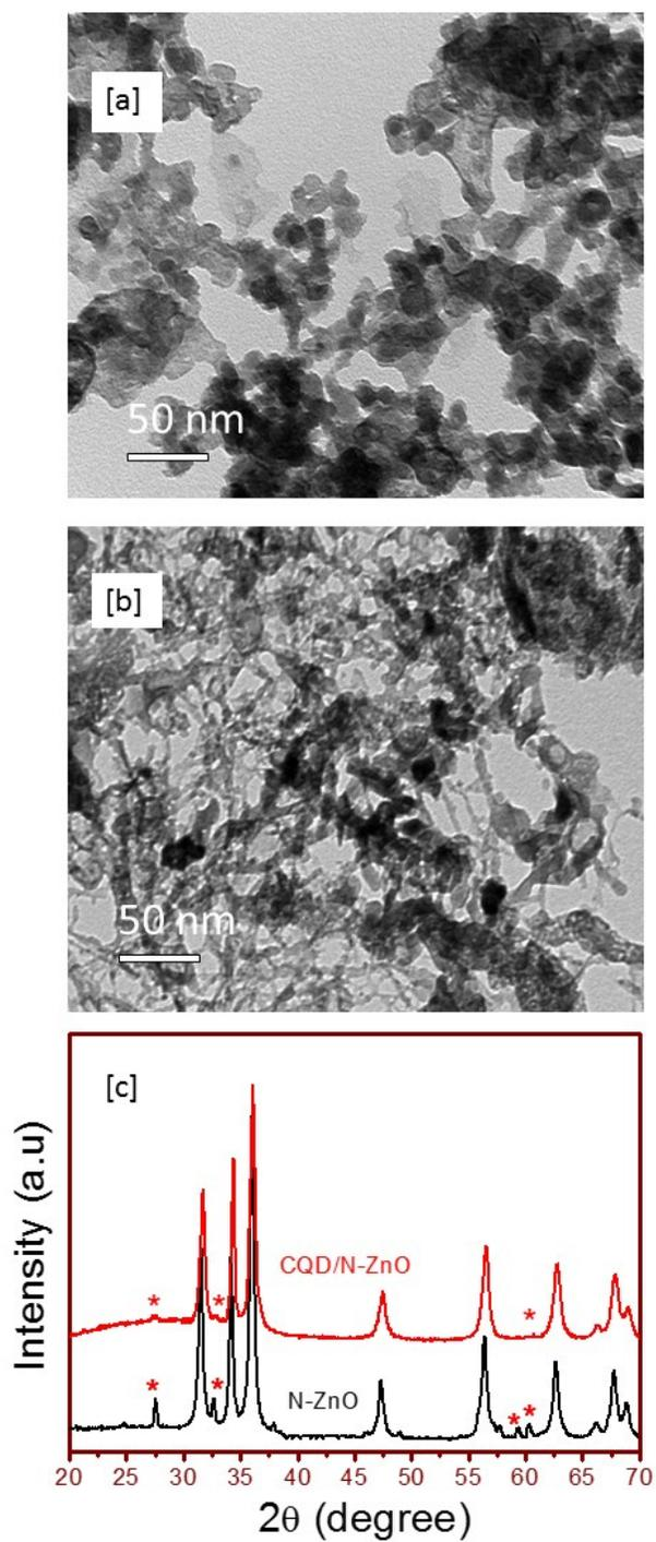
Figure S7. TEM images of (a) CQD/N-ZnO and (b) N-doped ZnO photocatalysts after 4<sup>th</sup> successive photocatalytic experiments and their respective (c) XRD spectra.
