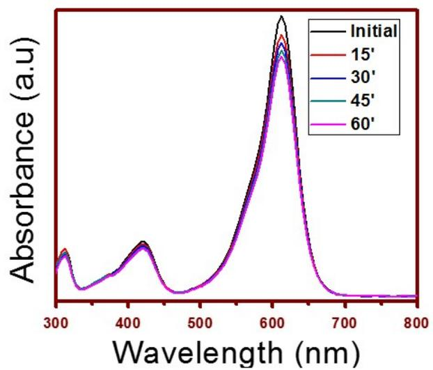
Figure S3. Photocatalytic degradation of MG dye solution under daylight irradiation without catalyst.
