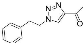
White solid; mp 110–112°C (lit: 114-115 °C); FT-IR (neat):  $\nu = 1683 \text{ cm}^{-1}$ ; <sup>1</sup>H NMR (400 MHz, CDCl<sub>3</sub>):  $\delta$  (ppm) 7.76 (s, 1H), 7.29-7.22 (m, 3H), 7.08-7.06 (m, 2H), 4.62 (t,  $J = 8.0 \text{ Hz}$ , 2H), 3.21 (t,  $J = 8 \text{ Hz}$ , 2 H), 2.64 (s, 3H); <sup>13</sup>C NMR (100 MHz CDCl<sub>3</sub>):  $\delta$  (ppm) 192.9, 147.9, 136.5, 129.0, 128.7, 127.5, 125.7, 52.0, 36.6, 27.2.
