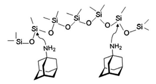
Fig. S3. Schematic presentation of arrangement of structure directing agent 1-adamantanamine in Silica backbone in zeolitic pores
