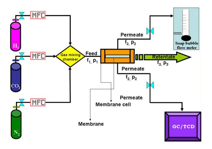
Fig S1 Schematic representation of permeation apparatus for the measurement of both single gas and mixed gas permeation.
