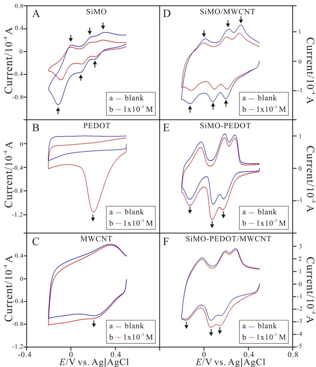
**Fig. S2** Cyclic voltammograms of (A) SiMO, (B) PEDOT, (C) MWCNT, (D) SiMO/MWCNT, (E) SiMO-PEDOT, and (F) SiMO-PEDOT/MWCNT modified GCEs examined in sulphuric solution (pH 1.5) containing  $[Na_2S_2O_8] =$  (a) blank and (b)  $1 \times 10^{-3}$  M, respectively. Scan rate =  $0.1 \text{ Vs}^{-1}$ .
