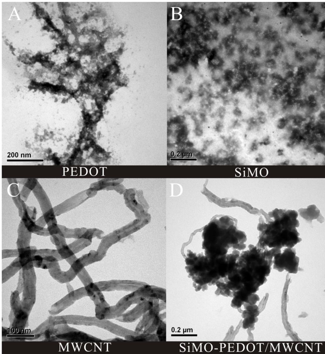
**Fig. S1** TEM images of (A) PEDOT, (B) SiMO, (C) MWCNT, and (D) SiMO-PEDOT/MWCNT coated Cu-net (300 mesh regular grid).
