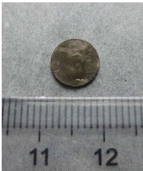
Figure S7. Digital photographs of the cold-pressed, free-standing \text{Ti}_4\text{AlN}_3 disc with a diameter of 8 mm and a thickness about 0.5 mm. The resistivity of disc, measured by a four-probe tester, is only ca. 1.4 \, \Omega/\square , indicating the good conductivity of this material.
