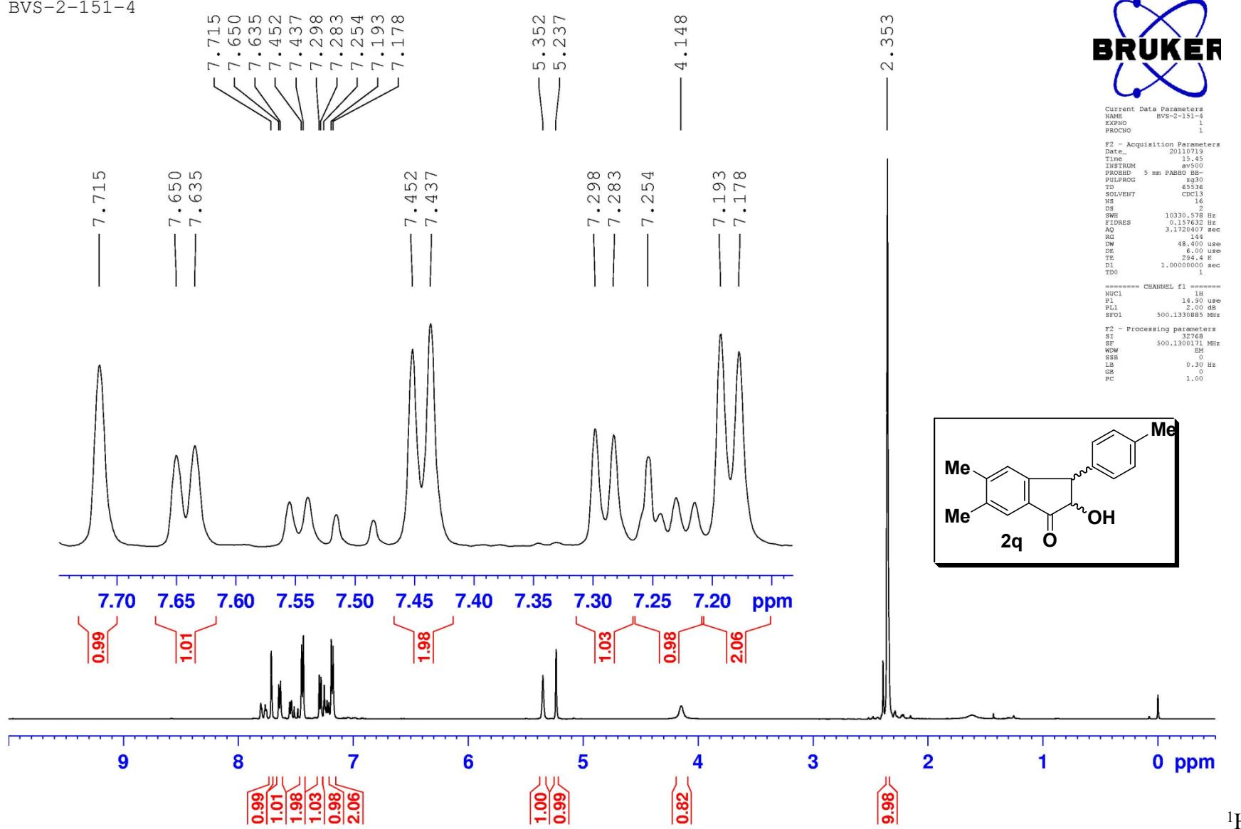
NMR (500 MHz,  $\text{CDCl}_3$ ) Spectrum of **2q**
