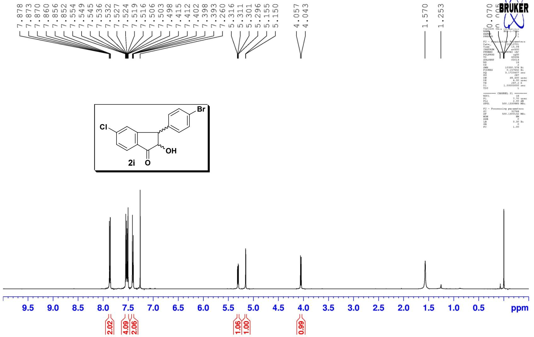
NMR (500 MHz,  $\text{CDCl}_3$ ) Spectrum of **2i**
