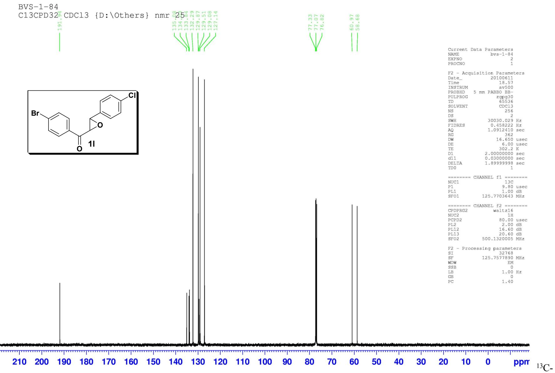
NMR (125 MHz,  $\text{CDCl}_3$ ) Spectrum of **11**
