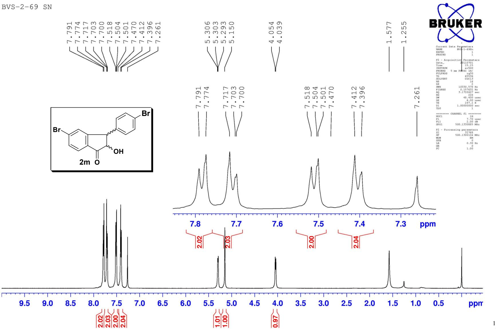
NMR (500 MHz, CDCl<sub>3</sub>) Spectrum of **2m**
