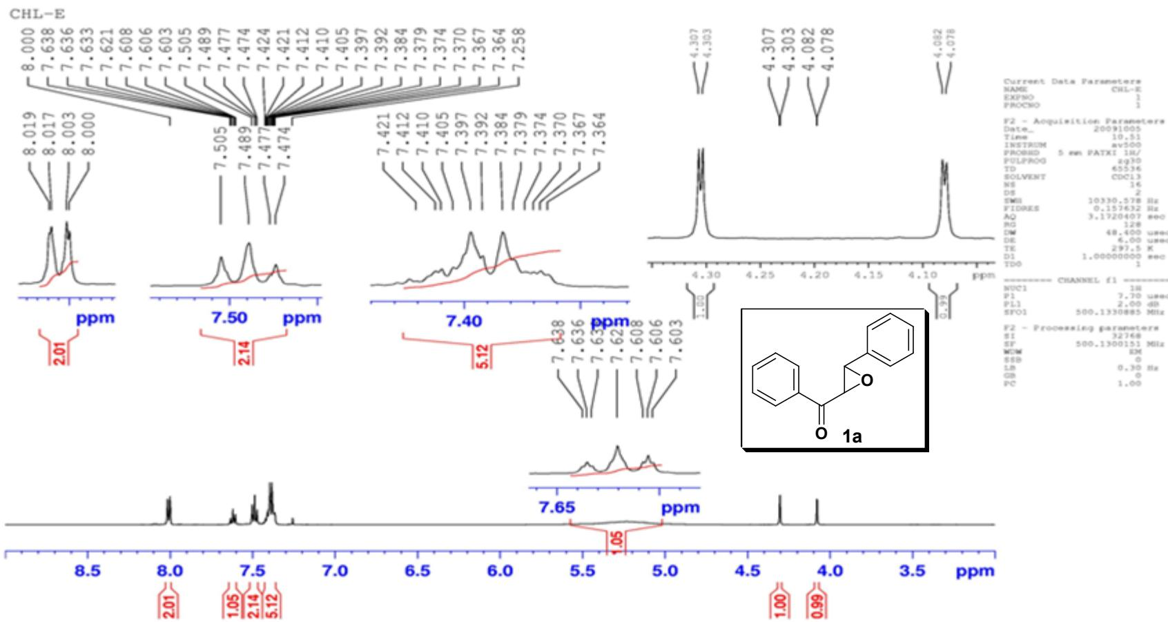
$^1\text{H}$ -NMR (500 MHz,  $\text{CDCl}_3$ ) Spectrum of **1a**
