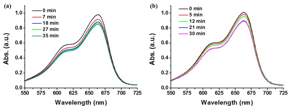
**Fig. S5** Absorption spectra of the reduction of MB in aqueous solution in the presence of (a) AC and (b) no catalyst.
