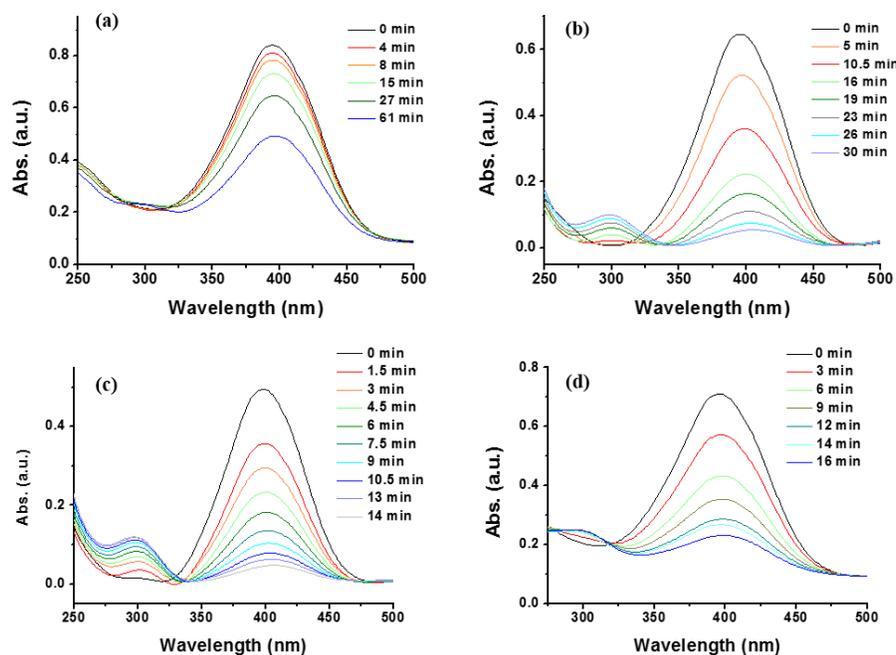
**Fig. S4** UV-vis spectra of the reduction of 4-nitrophenol in aqueous solution with the catalysts (a) Pd/AC-noCD, (b) Pd/AC(no wash), (c) Pd/AC-1, and (d) Pd/AC-2.
