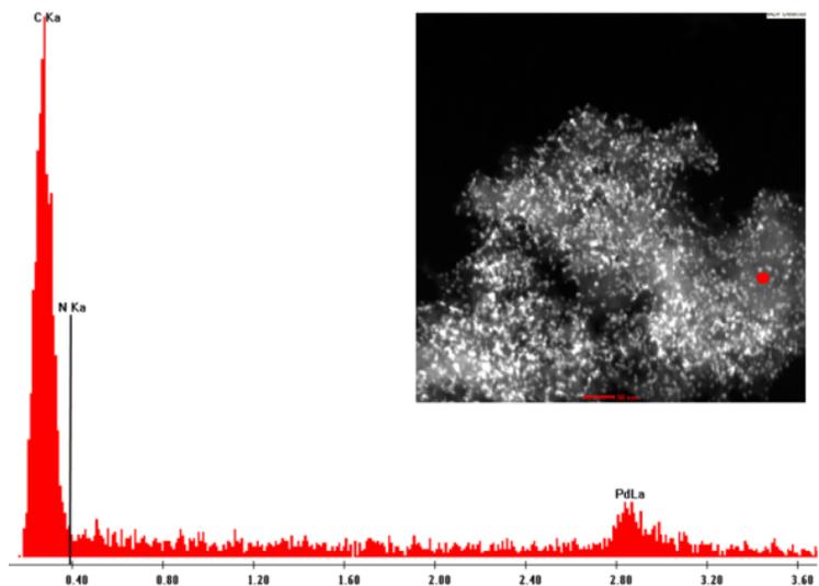
**Fig. S3** EDS spectrum of the area marked as a small red spot in the corresponding dark-field image of the sample Pd/AC(wash).
