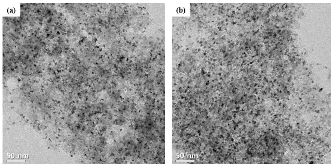
**Fig. S2** TEM images of the samples (a) Pd/AC(no wash) and (b) Pd/AC(wash).
