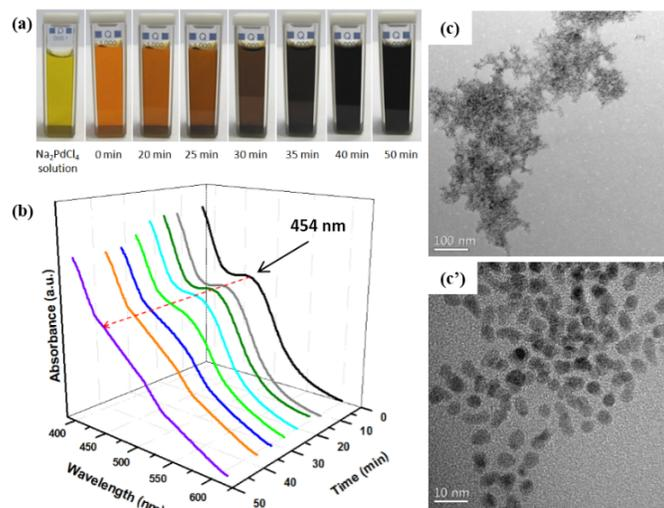
**Fig. S1** (a) Digital photographs of the mixture containing  $\text{Na}_2\text{PdCl}_4$ , AA, and CD at various reaction times; (b) Time evolution of the UV-vis absorption spectra of the mixture; (c) and (c') TEM images of CD-stabilized Pd nanoparticles after 45 minutes at two different magnifications.
