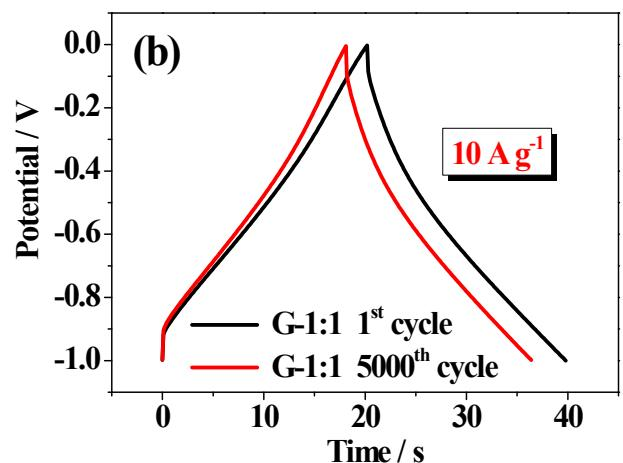
**Fig. S6.** G-1:1 carbon sample: (a) cycling stability measured at  $10 \text{ A g}^{-1}$ ; (b) GCD curves before/after 5000<sup>th</sup> cycles cycling stability measured at  $10 \text{ A g}^{-1}$ .
