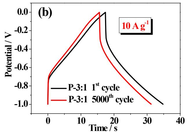
**Fig. S2.** P-3:1 carbon sample: (a) cycling stability measured at  $10\text{ A g}^{-1}$ ; (b) GCD curves before/after  $10^4$ cycles cycling stability measured at  $10\text{ A g}^{-1}$ .
