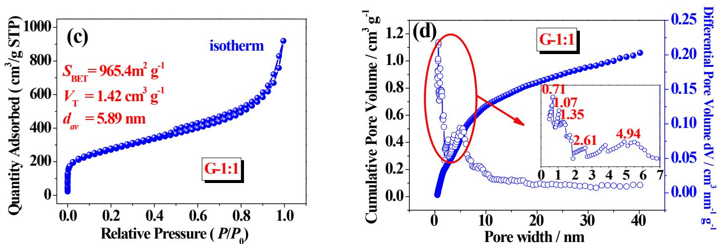
**Fig. S3.** The G-1:1 sample: (a-b) HRTEM images as well as the magnified SAED pattern (the insets); (c) N<sub>2</sub> adsorption-desorption isotherm; (d) cumulative pore volume and pore size distribution curves (estimated by using a slit/cylindrical NLDFT model).
