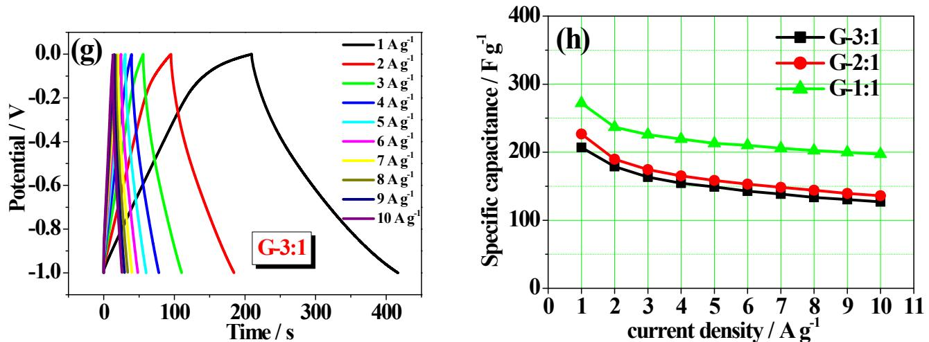
**Fig. S5. G-1:1, G-2:1, G-3:1** carbon samples: (a, b, c) CV curves; (d) specific capacitances calculated from CV curves; (e, f, g) GCD curves; (h) specific capacitances calculated from GCD curves.
