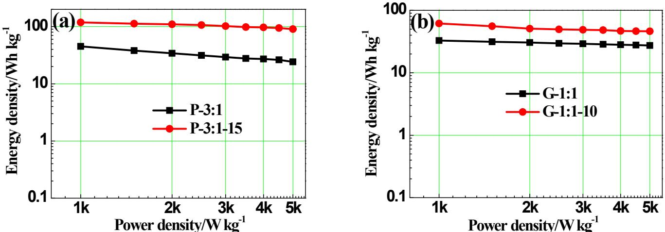
**Fig. S7.** Ragone plots showing energy density vs. power density: (a) The **P-3:1**, **P-3:1-15** samples; (b) The **G-1:1**, **G-1:1-10** samples.
