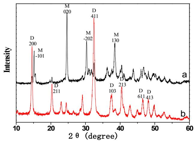
Fig. S2. XRD of CaOx samples obtained in the presence of casein with different concentrations,  $[\text{CaCl}_2] = 5 \text{ mM}$ ,  $[\text{casein}] = 0.2 \text{ g L}^{-1}$  (a) and  $6 \text{ g L}^{-1}$  (b).
