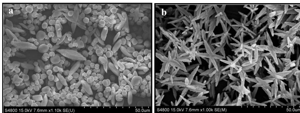
Fig. S3. SEM images of CaOx samples obtained in the presence of 4.0 g L<sup>-1</sup> casein at (a) pH 10.5 and (b) pH 3.5, [CaCl<sub>2</sub>] =5 mM.
