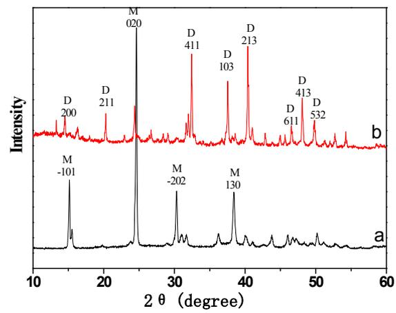
Fig. S4. XRD pattern of CaOx samples obtained in the presence of  $4.0 \text{ g L}^{-1}$  casein at (a) pH 3.5 and (b) pH 10.5,  $[\text{CaCl}_2] = 5 \text{ mM}$ .
