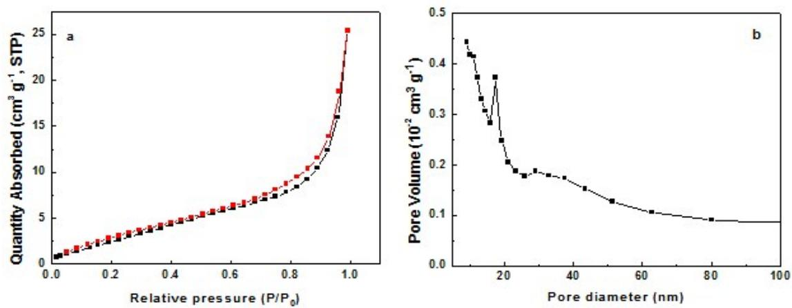
Fig. S6. Nitrogen adsorption-desorption isotherms (A) and Pore-size distribution curves of the double cashew-shaped CaOx.
