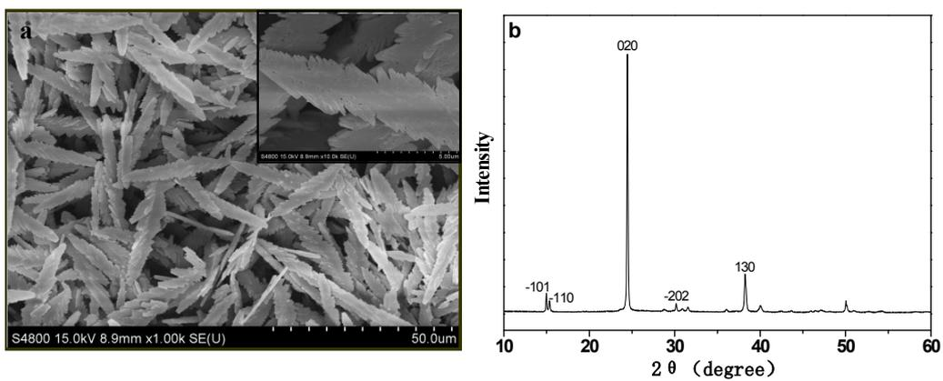
Fig. S1. SEM image (a) and XRD pattern (b) of CaOx obtained in the absence of casein at  $25 \pm 1$  °C,  $[\text{CaCl}_2] = 5$  mM.
