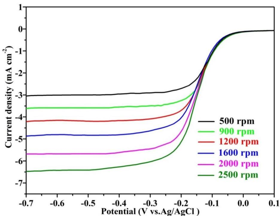
**Fig. S6** Linear sweep voltammetry curves of the commercial Pt/C in an O<sub>2</sub>-saturated 0.1 M NaOH solution at a sweep rate of 10 mV s<sup>-1</sup> under various rotation rates.
