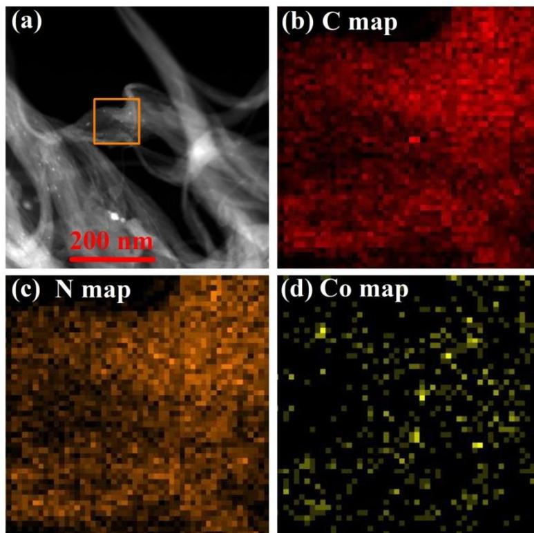
**Fig. S1** (a) Scanning transmission electron microscopy (STEM) image of Co-g- $\text{C}_3\text{N}_4$  on SWCNTs. The corresponding element mapping images of (b) carbon, (c) nitrogen and (d) cobalt of the Co-g- $\text{C}_3\text{N}_4$ /SWCNTs composite, indicating the homogeneous distribution of Co-g- $\text{C}_3\text{N}_4$  on SWCNTs.
