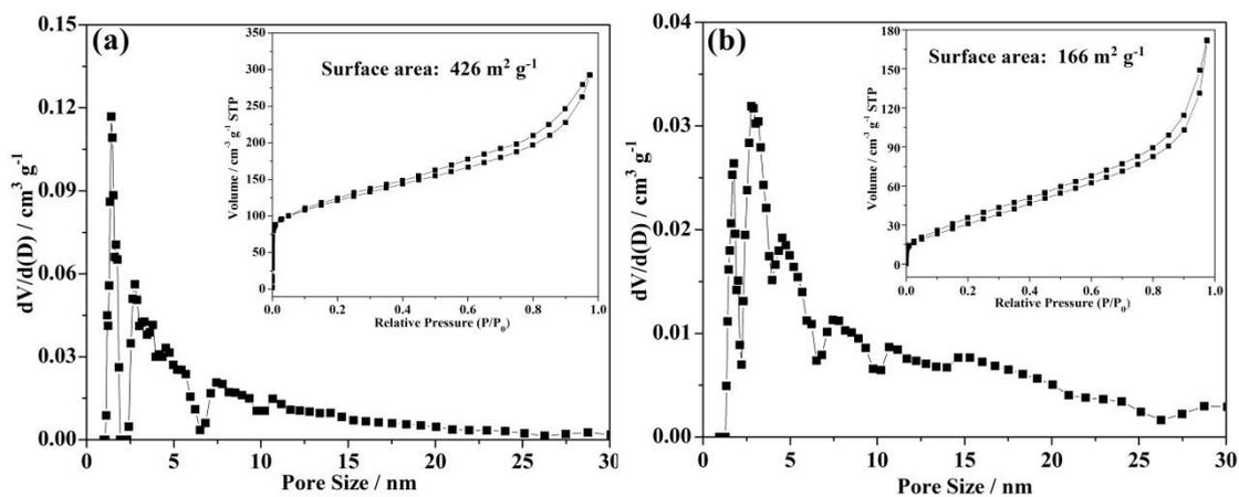
**Fig. S3** The pore-size distribution curve: (a) Co-g-C<sub>3</sub>N<sub>4</sub>/SWCNTs. Inset: the nitrogen adsorption isotherm of Co-g-C<sub>3</sub>N<sub>4</sub>/SWCNTs; (b) Pure-SWCNTs. Inset: the nitrogen adsorption isotherm of Pure-SWCNTs.
