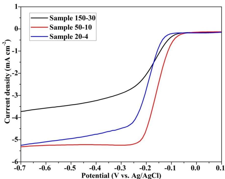
**Fig. S7** LSV curves of Co-g-C<sub>3</sub>N<sub>4</sub>/SWCNTs with varying proportions in an O<sub>2</sub>-saturated 0.1 M NaOH solution at a sweep rate of 10 mV s<sup>-1</sup> and 1600 rpm.
