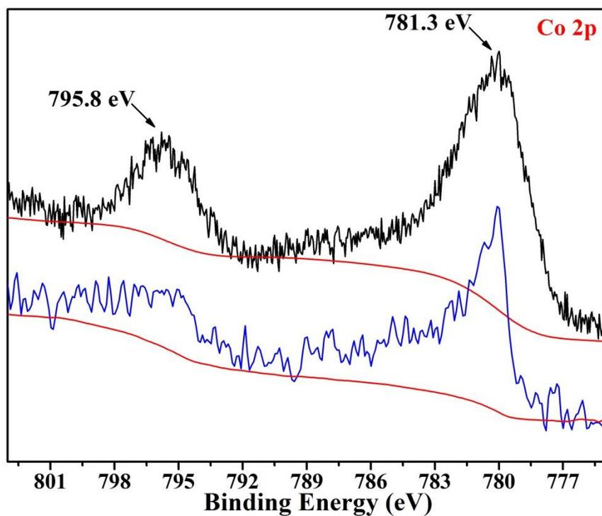
**Fig. S4** The XPS survey spectra of Co 2p spectrum: Co-g-C<sub>3</sub>N<sub>4</sub>/SWCNTs (**black curves**) and the Co-g-C<sub>3</sub>N<sub>4</sub>/SWCNTs composites washed by excess HCl solution (**blue curves**).
