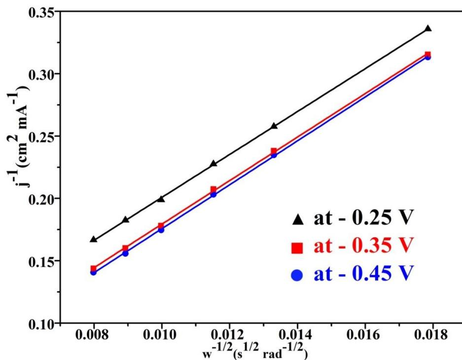
**Fig. S8** Koutecky-Levich plots at different potentials for ORR in an O<sub>2</sub>-saturated 0.1 M NaOH solution for Co-g-C<sub>3</sub>N<sub>4</sub>/SWCNTs.
