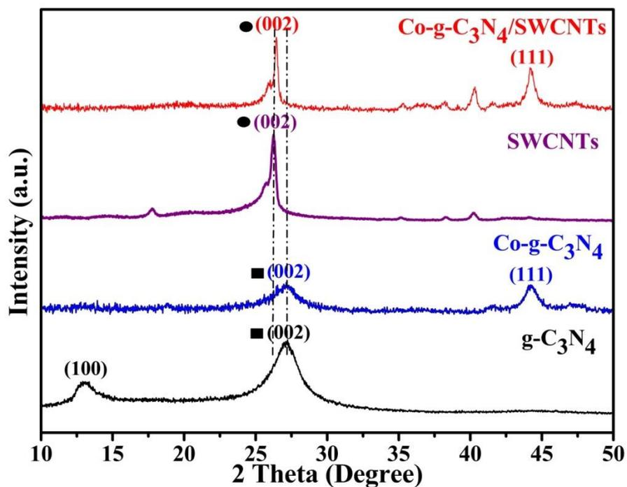
**Fig. S2** The XRD patterns of Co-g- $\text{C}_3\text{N}_4$ /SWCNTs in comparison to g- $\text{C}_3\text{N}_4$ , Co-g- $\text{C}_3\text{N}_4$ , and SWCNTs.
