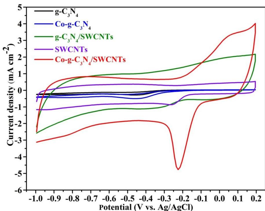
**Fig. S5** Cyclic voltammograms of g-C<sub>3</sub>N<sub>4</sub>, Co-g-C<sub>3</sub>N<sub>4</sub>, SWCNTs, g-C<sub>3</sub>N<sub>4</sub>/SWCNTs, and Co-g-C<sub>3</sub>N<sub>4</sub>/SWCNTs with a scan rate of 50 mV s<sup>-1</sup> in an O<sub>2</sub>-saturated 0.1 M NaOH solution.
