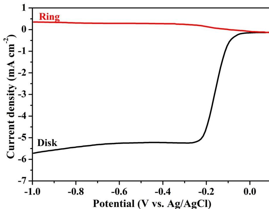
**Fig.S9** RRDE voltammogram curves of Co-g-C<sub>3</sub>N<sub>4</sub>/SWCNTs catalyst at the rotation speed of 1600 rpm.
