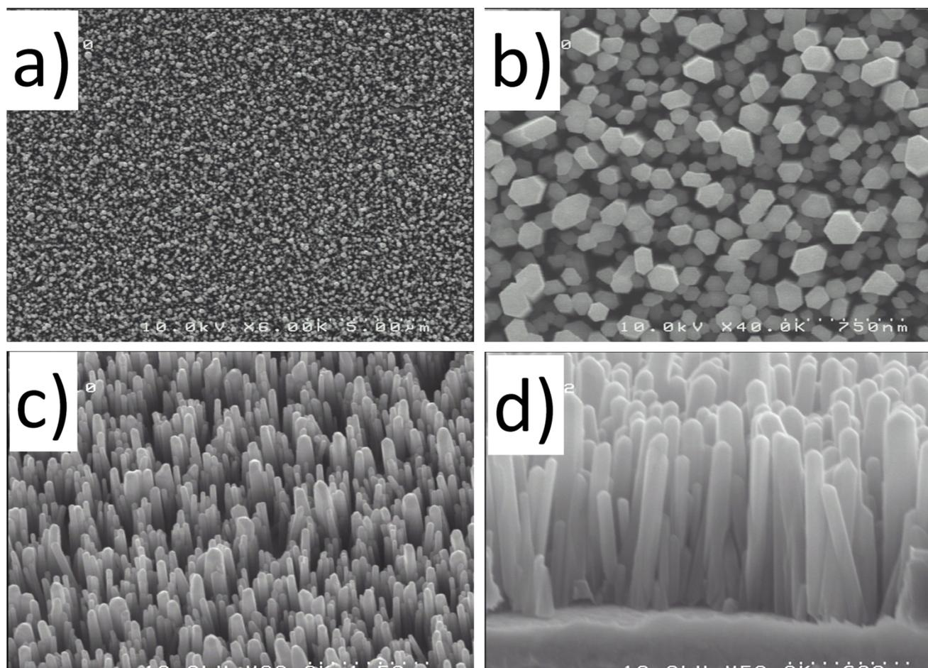
**Figure S1** A collection of Scanning electron microscope images of as-grown ZnO NW arrays on Au coated Si substrates. a-b) top-view images at various magnifications, c) SEM image at  $\sim 30^\circ$  tilt, d) cross-sectional image of the ZnO NWs.
