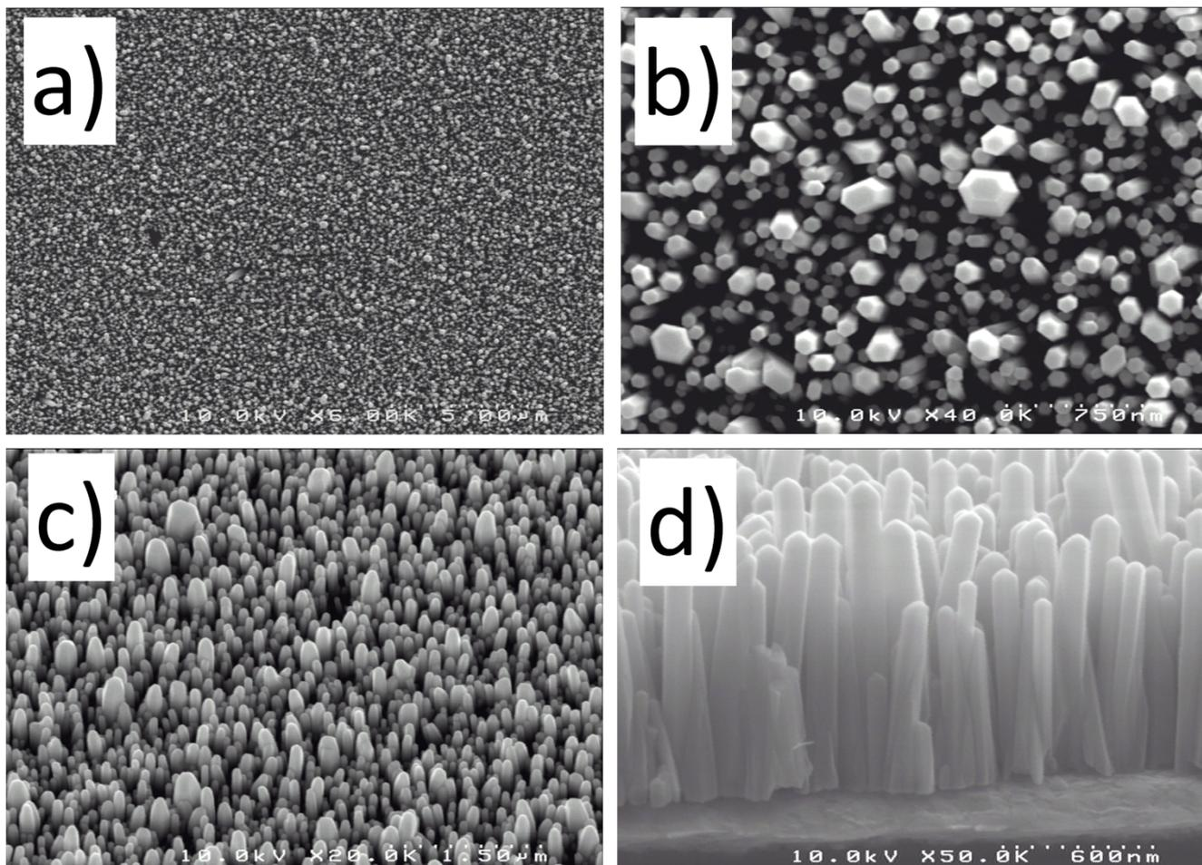
**S3** A collection of Scanning electron microscope images of the ZnO NWs on Au coated Si substrates after 450°C thermal annealing in ambient air. a-b) top-view images at various magnifications, c) SEM image at ~30° tilt, d) cross-sectional view of the ZnO NWs
