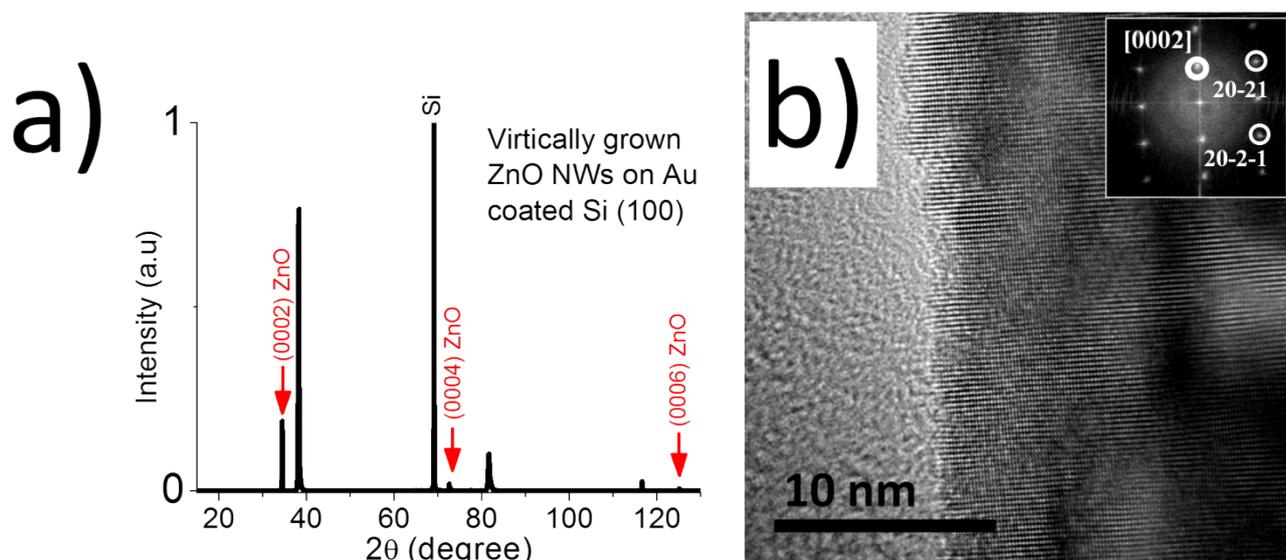
**Figure S2** a) x-ray diffraction data and b) high resolution transmission electron microscope image of a representative ZnO NW on Au coated Si substrates.
