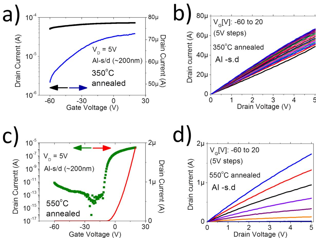
**Figure S5** a-b) Transfer and output scans for the 350°C annealed single ZnO nanowire device. c-d) transfer and output scans for 550°C thermally annealed ZnO nanowire device.
