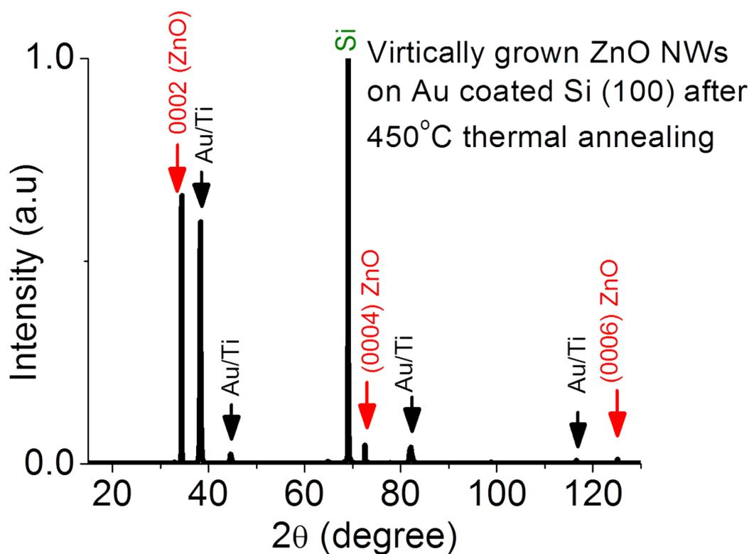
**Figure S4** a) x-ray diffraction data for ZnO NW arrays on a Au coated Si substrate after 450°C thermal annealing under ambient air conditions.
