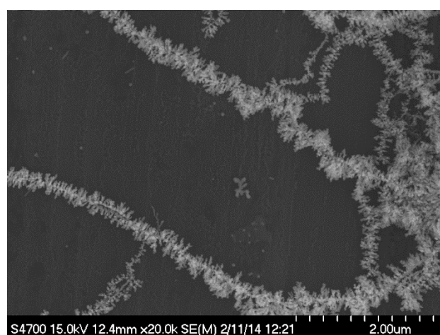
Fig S10 SEM images of one-dimensional Au nanomaterials synthesized by using CTAB (3.5 mM) and PVP (0.5 mM) as the capping agents at 25 °C; (a) lower magnification and (b) higher magnification images. The concentration of H Au Cl 4 , PEG is 2.0 mM and 0 mM, respectively. The circled areas in Fig. S10a show that the Al substrate is etched after Au atoms deposit on the top surface of Al. A trace of products are also found of the bottom of Al substrate.
