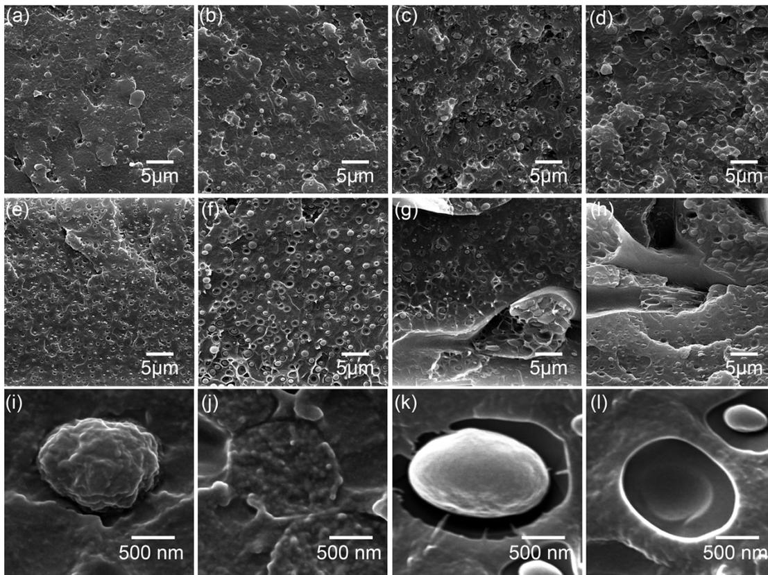
Fig. S2. The SEM images of the SPEEK/PVDF-g-PSSA blend membranes at the PVDF-g-PSSA content of (a) 5 wt. %, (b) 10 wt. %, (c) 15 wt. %, and (d) 20 wt. %; the SEM images of the SPEEK/PVDF blend membranes at the PVDF content of (e) 5 wt. %, (f) 10 wt. %, (g) 15 wt. %, and (h) 20 wt. %; (i) and (j) high-magnification SEM images of the SPEEK/PVDF-g-PSSA (20 wt. %) membrane; (k) and (l) high-magnification SEM images of the SPEEK/PVDF (20 wt. %) membrane
