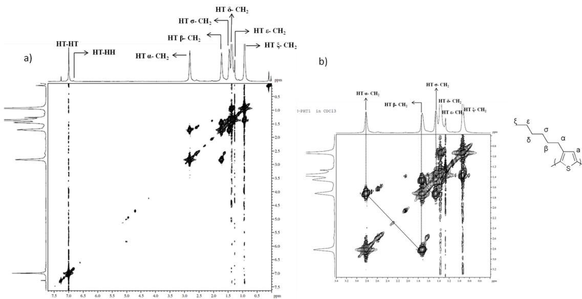
Figure S2. COSY NMR of Poly (3-hexyl thiophene) **1**, (a) Full spectra, (b) expanded.
