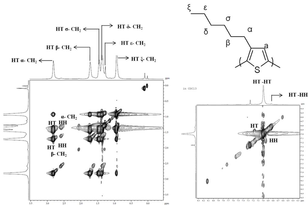
**Figure S8.** TOCSY NMR Spectra of Poly (3-hexyl thiophene) **1** (Expanded).
