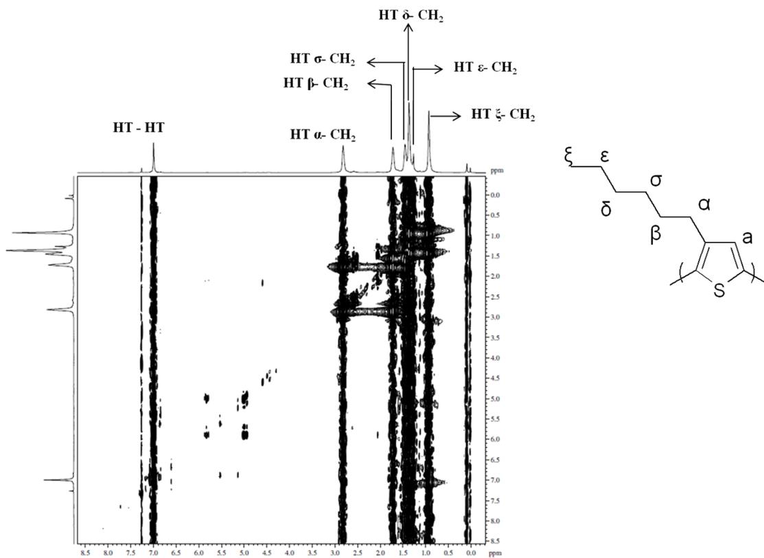
**Figure S3.** Double Quantum Filtered COSY NMR of Poly (3-hexyl thiophene) **1**.
