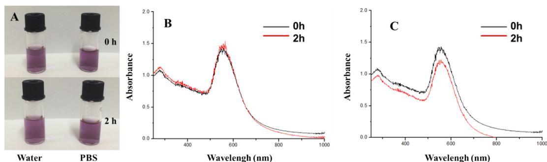
**Fig. S4. (A) Photo of polydopamine encapsulated SERS probes before and after 2 hours store. (B) UV/Vis spectra of polydopamine encapsulated SERS probes before and after 2 hours store in water. (C) UV/Vis spectra of polydopamine encapsulated SERS probes before and after 2 hours store in PBS buffers.**
