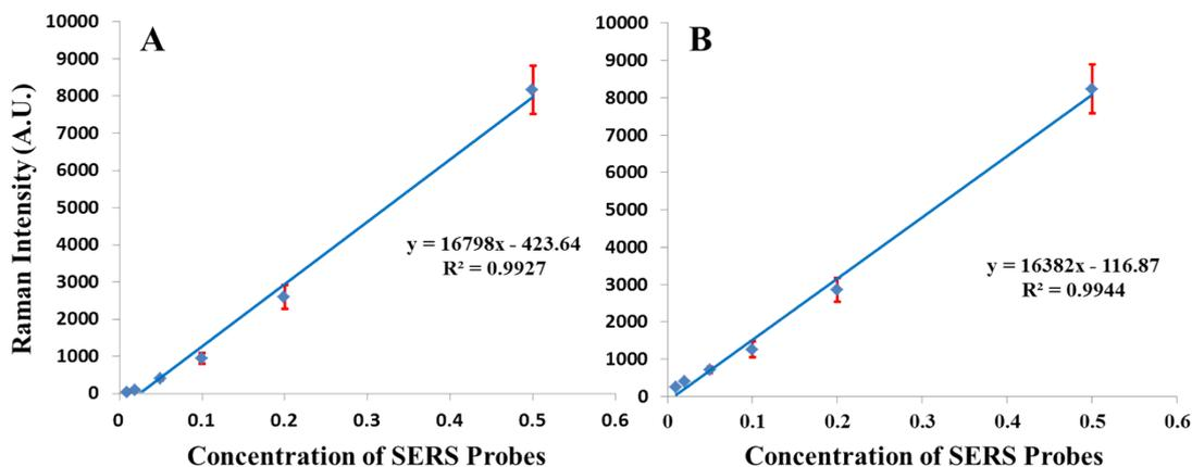
**Fig. S6.** Regression analysis of the SERS intensity of SERS probes (at  $1080\text{ cm}^{-1}$ ) versus the SERS probes concentration in water (A) and PBS (B).
