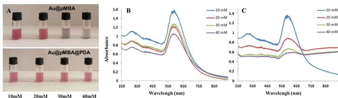
**Fig. S3. (A) Color changes of Au colloid with and without the encapsulation of polydopamine in various salt concentration. (B) UV/Vis spectra of polydopamine**
