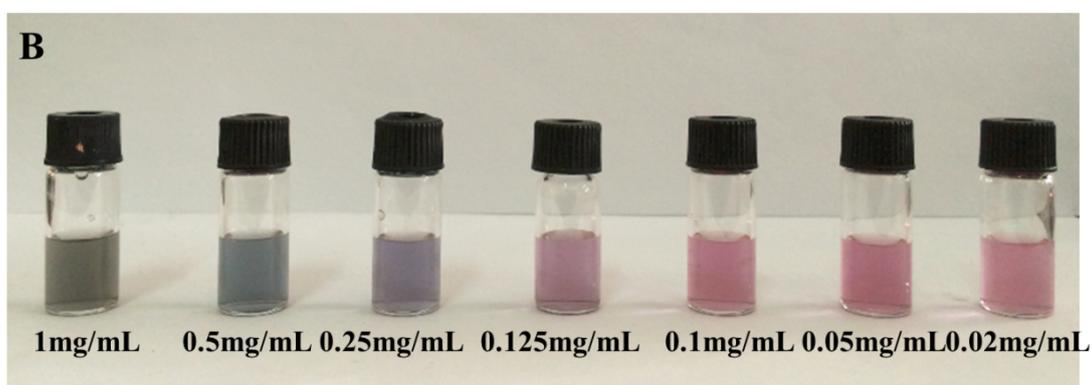
**Fig. S1 (A)** SERS spectrum of polydopamine coated SERS nano tags synthesized under different dopamine concentration. **(B)** Photo of polydopamine coated SERS nano tags synthesized under different dopamine concentration.
