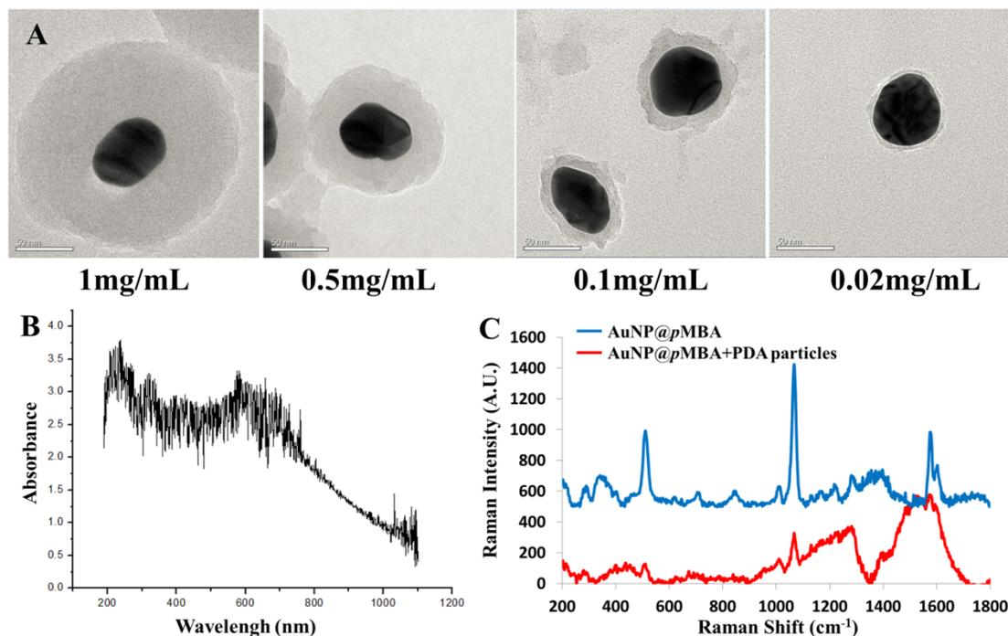
**Fig. S2** (A) TEM images of polydopamine encapsulated SERS probes under different concentrations of dopamine. (B) UV/Vis spectra of self-polymerization dopamine particles generated by the self-polymerization of 1 mg/mL dopamine in 10 mM Tris-HCl buffer (pH 8.5). (C) Raman spectra of SERS active nano tags (Au NPs@pMBA) before and after self-polymerization dopamine particles addition.
