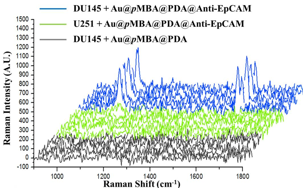
**Fig. S7.** SERS spectra of DU145 cells incubated with antibody modified SERS probes (blue), U251 cells incubated with antibody modified SERS probes (green) and DU145 cells incubated with negative control SERS probes (gray).
