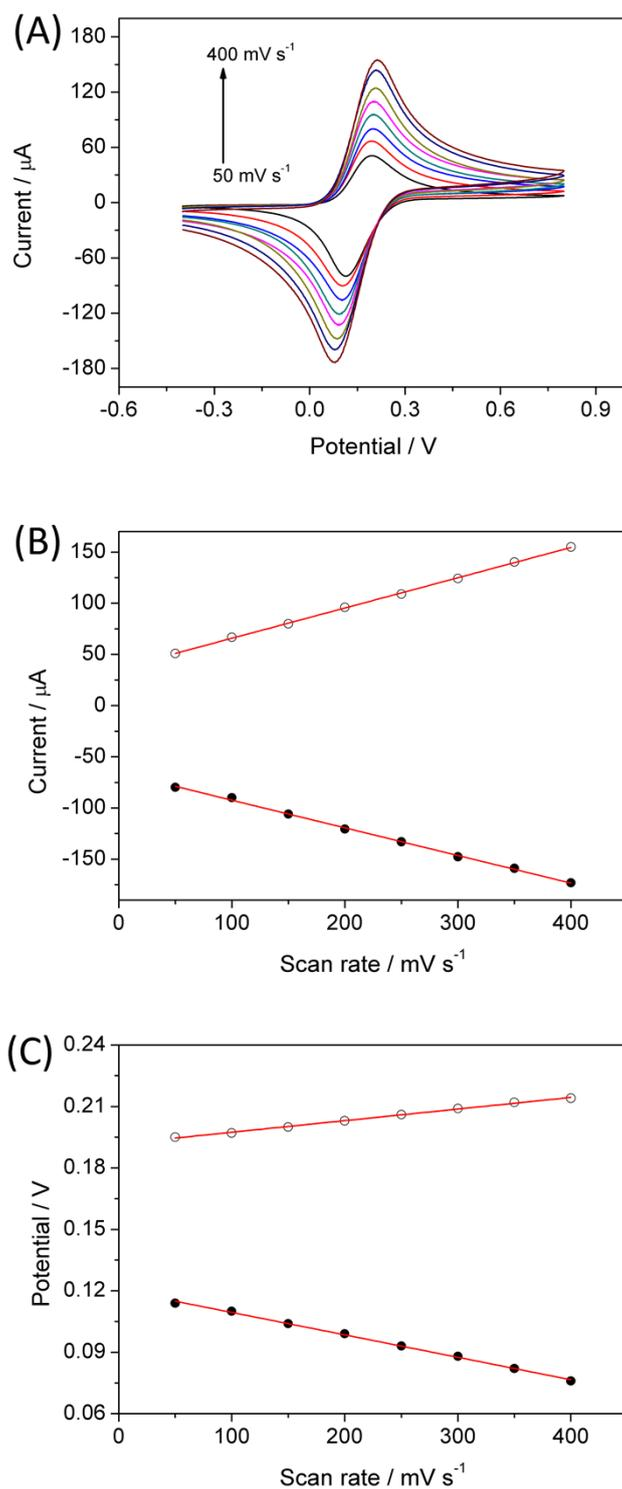
**Fig. S2.** CV studies of SS-β-CD-Pd@RGO/GCE as a function of scan rate (50–400 mV s<sup>-1</sup>) using 2.0 mM [Fe(CN)<sub>6</sub>]<sup>3-/4-</sup> redox couple (1:1) with 0.1 M KCl as supporting electrolyte (A); Magnitude of current response vs. scan rate (B); Value of redox potential vs. scan rate (C).
