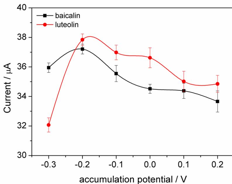
**Fig. S9.** Effect of accumulation potential on the oxidation peak currents of 20.0  $\mu\text{M}$  baicalin and 10.0  $\mu\text{M}$  luteolin at SS- $\beta$ -CD-Pd@RGO/GCE in 0.1 M pH 3.0 PBS by DPV. Pulse width: 0.05 s; amplitude: 0.05 V.
