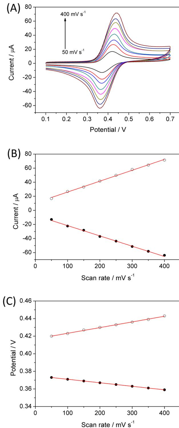
**Fig. S4** (A) CVs obtained for 10  $\mu\text{M}$  luteolin at SS- $\beta$ -CD-Pd@RGO/GCE in 0.1 M PBS (pH 3.0) at various scan rates: 50, 100, 150, 200, 250, 300, 350, and 400  $\text{mV s}^{-1}$ ; (B) Magnitude of redox peak currents vs. scan rate; (C) Value of redox peak potentials vs. scan rate.
