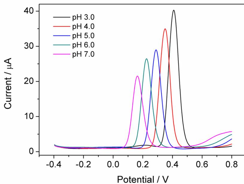
**Fig. S6.** Effect of detection medium pH on the oxidation peak currents of 10 μM of luteolin at SS-β-CD-Pd@RGO/GCE in 0.1 M pH 3.0 PBS.
