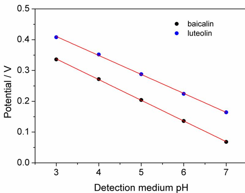
**Fig. S7.** Variation of the peak potentials of baicalin and luteolin vs. pH of the detection medium.
