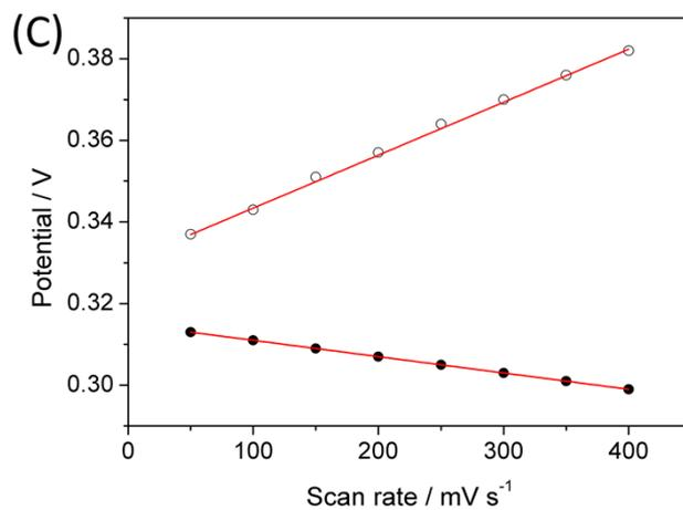
**Fig. S3** (A) CVs obtained for 20  $\mu\text{M}$  baicalin at SS- $\beta$ -CD-Pd@RGO/GCE in 0.1 M PBS (pH 3.0) at various scan rates: 50, 100, 150, 200, 250, 300, 350, and 400  $\text{mV s}^{-1}$ ; (B) Magnitude of redox peak currents vs. scan rate; (C) Value of redox peak potentials vs. scan rate.
