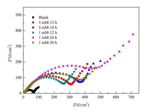
**Fig. S1** Nyquist plots in 0.5 M HCl for the blank copper and OP covered copper electrodes immersed in 1.0 and 5.0 mM OP solution for different time
