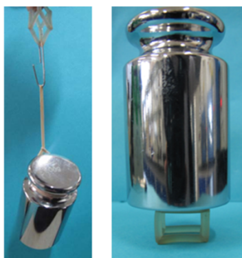
Figure S5. The cubic device constructed using MD50 copolymer elastomer can bear load of 500g (comparable to 400 times the weight of itself ) without failure.
