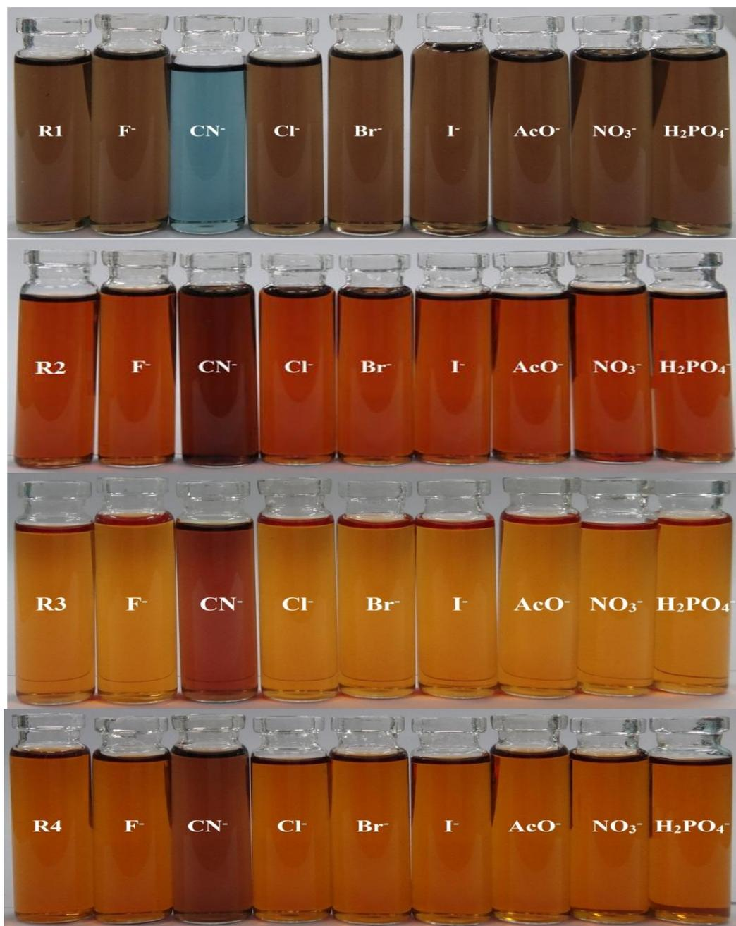
**Figure S2.** Color changes observed in DMF solution of **R1-R4** ( $6.25 \times 10^{-4}$  M) upon addition of various anions.
