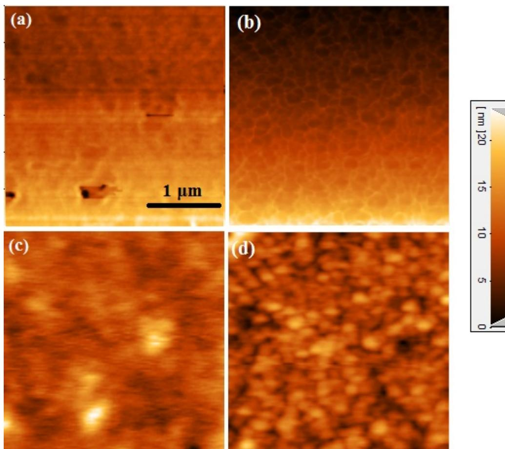
Fig. S2 AFM topographical images of (a) pure PEDOT-PSS, (b) CuTSPc@3D-(N)GFs/PEDOT-PSS and phase images of (c) pure PEDOT-PSS and (d) CuTSPc@3D-(N)GFs/PEDOT-PSS nanocomposite sensing films.
