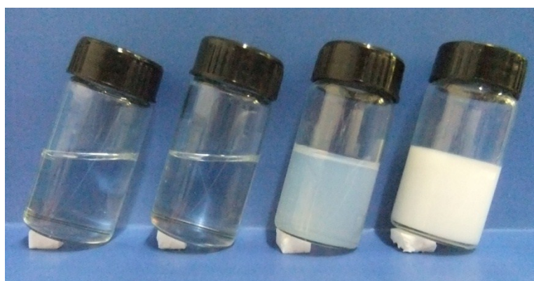
Figure S2 (a) citric acid/ethanol solution; (b) \text{ZrOCl}_2 \cdot 8\text{H}_2\text{O} + \text{Y}(\text{NO}_3)_3 \cdot 6\text{H}_2\text{O} ethanol solution; (c) mixture of 1 ml citric acid ethanol solution and 10 ml \text{ZrOCl}_2 \cdot 8\text{H}_2\text{O} + \text{Y}(\text{NO}_3)_3 \cdot 6\text{H}_2\text{O} ethanol solution (d) mixture of 9 ml citric acid ethanol solution and 10 ml \text{ZrOCl}_2 \cdot 8\text{H}_2\text{O} + \text{Y}(\text{NO}_3)_3 \cdot 6\text{H}_2\text{O} ethanol solution .
