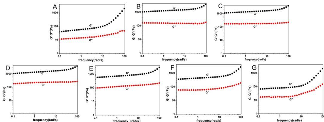
**Fig. S-6.** Rheological measurement with the mode of dynamic frequency sweep at the frequency of 1 rad/s and strain of 0.5% for the gel of Nap-FFYK-CA with different equivalent of vancomycin: A (0.005 equiv.), B (0.01 equiv.), C (0.02 equiv.), D (0.05 equiv.), E (0.1 equiv.), F (0.2 equiv.), and G (0.3 equiv.).
