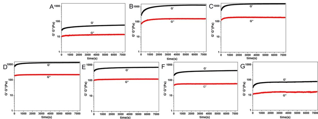
**Fig. S-5.** Rheological measurement with the mode of dynamic time sweep at the frequency of 1 rad/s and strain of 0.5% for the gels of Nap-GFFYEG<sup>D</sup>A<sup>D</sup>A with different equivalent of vancomycin: A (0.005 equiv.), B (0.01 equiv.), C (0.02 equiv.), D (0.05 equiv.), E (0.1 equiv.), F (0.2equiv.), and G (0.3 equiv.).
