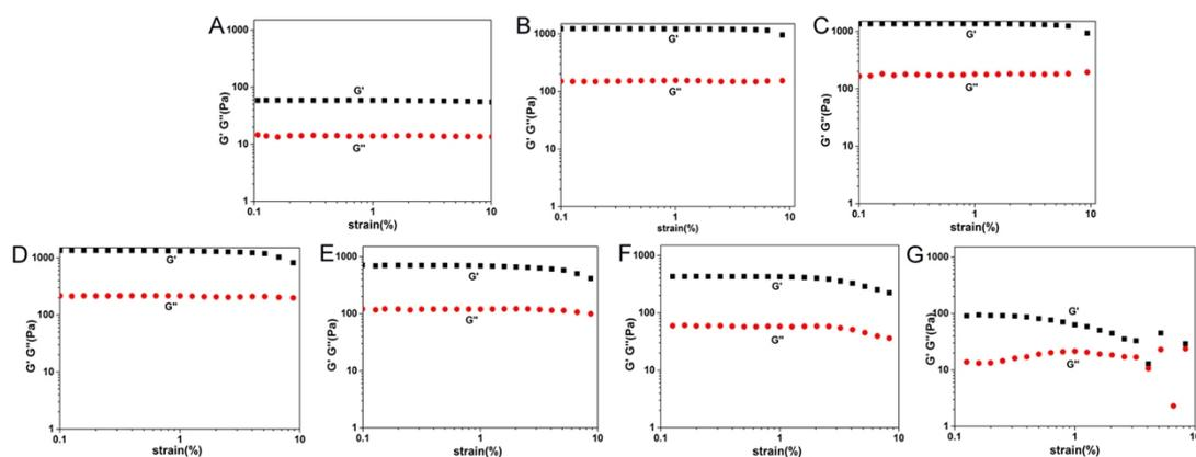
**Fig. S-7.** Rheological measurement with the mode of dynamic strain sweep at the frequency of 1 rad/s and strain of 0.1% for the gel of Nap-FFYGGK-CA with different equivalent of vancomycin: A (0.005 equiv.), B (0.01 equiv.), C (0.02 equiv.), D (0.05 equiv.), E (0.1 equiv.), F (0.2equiv.), and G (0.3 equiv.)
