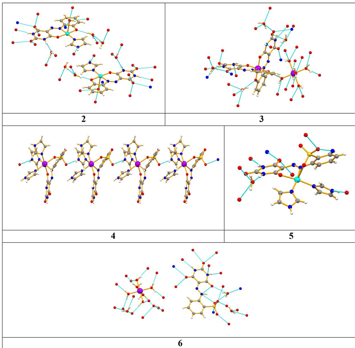
**Figure 10S.** Hydrogen bond interactions (in dashed blue lines; see also Table 3S) in 2–6. Only in 4 these contacts lead to infinite 1D chains; in all the other compounds such interactions give rise to 3D frameworks.
