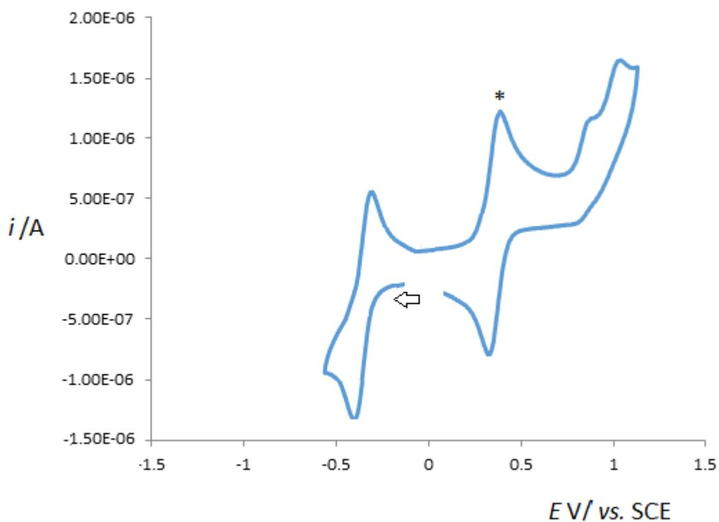
**Figure 14S.** Cyclic voltammogram, initiated by the cathodic sweep, of **3** in a 0.2 M  $[n\text{Bu}_4\text{N}][\text{BF}_4]/\text{NCMe}$  solution, at a Pt disc working electrode ( $d = 0.5$  mm), run at a scan rate of  $200 \text{ mVs}^{-1}$ . \*  $[\text{Fe}(\eta^5\text{-C}_5\text{H}_5)_2]^{0/+}$ .
