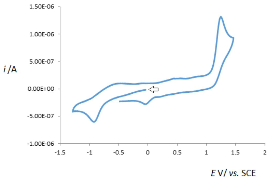
**Figure 11S.** Cyclic voltammogram, initiated by the cathodic sweep, of  $\text{H}_4\text{L}^1$  in a 0.2 M  $[\text{nBu}_4\text{N}][\text{BF}_4]/\text{NCMe}$  solution, at a Pt disc working electrode ( $d = 0.5$  mm), run at a scan rate of  $200 \text{ mVs}^{-1}$ .
