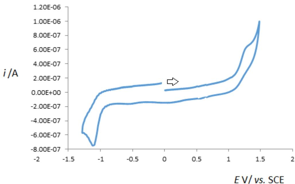
**Figure 12S.** Cyclic voltammogram, initiated by the anodic sweep, of **1** in a 0.2 M  $[\text{nBu}_4\text{N}][\text{BF}_4]/\text{NCMe}$  solution, at a Pt disc working electrode ( $d = 0.5$  mm), run at a scan rate of  $200 \text{ mVs}^{-1}$ .
